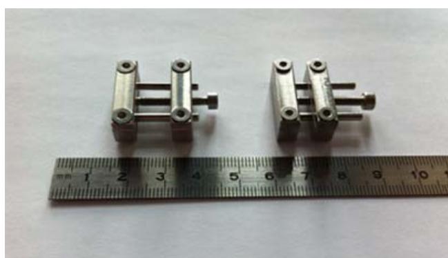
Figure S2: Devices used for the stretching of modified silicone sheets. The silicone sheets are placed between the two clamps and stretched manually.
