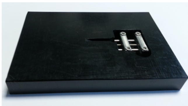
Figure 2.8: Homemade support elaborate to monitor the enzymatic activity using a spectrofluorimeter SAFAS (Xenius XC, SAFAS, Monaco).
