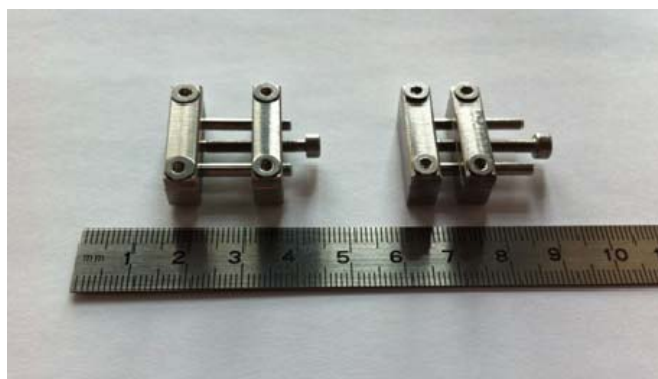
Figure S-1: Picture of the stretching devices. The silicone sheets are placed between the two clamps.
