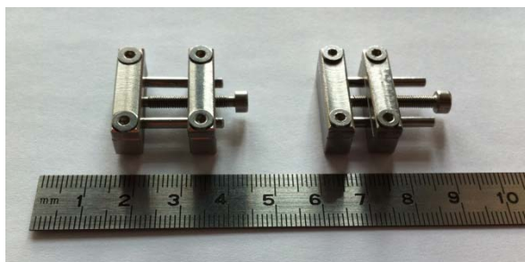
Figure 2.7: Stretching devices: The silicone sheets are placed between the two clamps and stretched manually.
