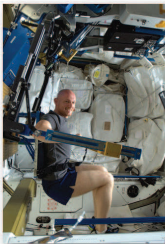
aRED : advanced Resistive Exercise Device
