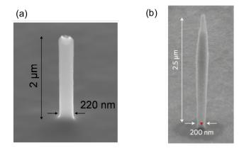
**Figure 2.11** – (a) scanning electron microscope images of fiber-like GaAs photonic wire [88]; (b) a single-photon source based on needle-like photonic wire made of GaAs embedding InAs QDs [19].
