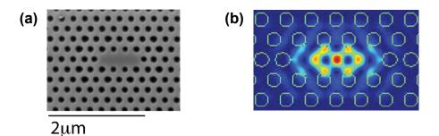
Figure 2.9 – Illustrations of the structure of photonic crystal cavity. (a) Scanning electron micrograph of the photonic crystal cavity in [82] showing a three-hole (L3) structure. (b) Simulated electric field intensity of the photonic crystal cavity [30].
