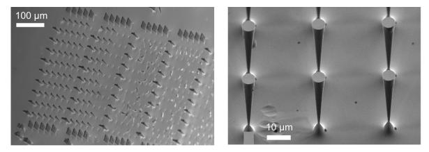
Figure B.2 – SEM images of giant trumpets. The maximum top diameter is 7  $\mu m$ .
