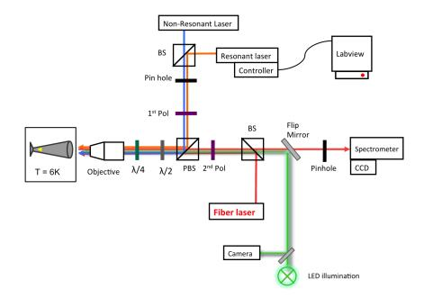
**Figure C.1** – Experimental setup of the resonant excitation with the presence of an intense fiber laser. The fiber laser has the energy much lower than the emission energy of the QD.
