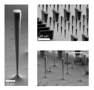
Figure 2.19 – Scanning electron microscope images of the trumpets - The sample contains several arrays of trumpets with top diameter ranging from 1  $\mu$ m to 4  $\mu$ m with the a step of 10 nm. The opening angle is fixed at 5°.
