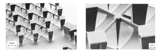
**Figure B.1** – Scanning electron microscope views of suspended trumpets. The top diameter ranges from 1.5 to 3.3  $\mu$ m with 20 nm step. The opening angle of the taper is 8.5°.
