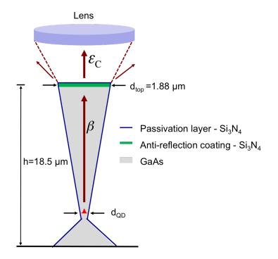
Figure 4.19 – Sketch of the trumpet in the measurement - The trumpet used in this study has the top facet diameter of 1.88  $\mu m$ , corresponds to a waist diameter around 550 nm where the QDs are located. The trumpet surface is covered with a 30 nm-thick Si<sub>3</sub>N<sub>4</sub> passivation layer.
