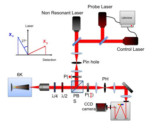
Figure 5.13 – Experimental setup of the two-mode giant non-linearity measurement - The same configuration as in chapter 4 is used. One more Toptica CW laser is added to the setup and it shares the path with other lasers toward the first pin hole and toward the sample. An ultra-weak non-resonant laser is always present in resonant excitation as explained in section 4.2.3.1. The cross-polarized detection is established with an angle 27° with respect to the  $X_x$  dipole polarization axis.
