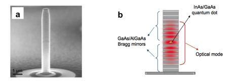
**Figure 2.8** – **Illustrations of the structure of a pillar microcavity -** (a) SEM image of the pillar microcavity described in [79]. (b) Sketch of a typical Qd-Pillar cavity system [80], a layer of self-assembled InGaAs QDs is embedded into a cavity and is sandwiched between two-distributed Bragg mirrors, inducing the confinement in lateral and vertical directions.
