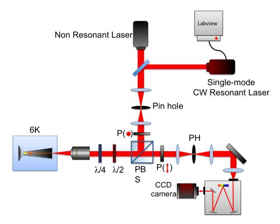
**Figure 4.6** – **Resonant excitation experimental setup -** A CW laser excites the QDs at a resonant frequency. The laser back-scattered light on the top surface of the trumpet induces a strong influence on the total signal detected by the CCD, thus a cross-polarized detection scheme is established to reject this laser background signal by using a polarizing beam-splitter.
