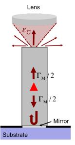
**Figure 2.16** – **Sketch of photon collection from quantum emitter embedded inside a finite photonic wire:** A mirror is integrated at the bottom to reflect upward the emission going to the bottom of the wire. The light exiting the top of the wire will be collected by an optical lens.
