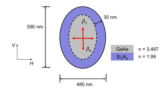
Figure 4.21 – Illustration of the cross-section at the QD-waist of the trumpet - The trumpet surface is covered with a 30 nm-thick  $Si_3N_4$  passivation layer, which results in the GaAs part dimensions 420 nm and 530 nm for respectively H and V directions. The refractive indices of GaAs and  $Si_3N_4$  are 3.487 and 1.99.
