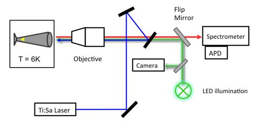
**Figure 3.14** – **Time-resolved PL experimental setup** - the QD is excited by a pulsed Ti:Sa laser, the emission from the QD is then sent to the spectrometer and collected by a single-photon photon counting module
