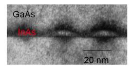
Figure 2.2 – TEM image of the cross section of the quantum dot structure - Selfassembled InAs/GaAs QDs are grown by Stranski-Krastanov method, strained InAs islands based on the wetting layer in GaAs matrix [47].
