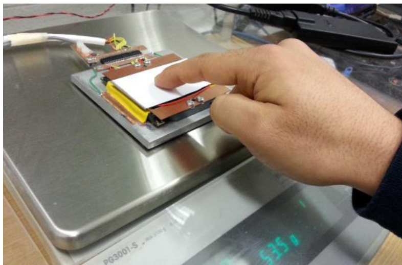
Figure 3.2: Experimental set-up of used to determine the tactile perception's threshold
