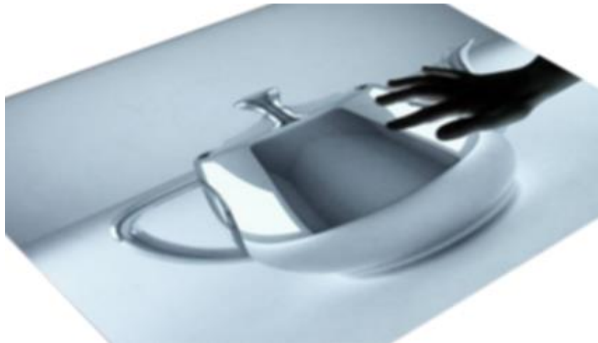
Figure 1-3: A developed tactile feedback device used to render 3D surfaces (Disney Research) by (Kim et al., 2013).
