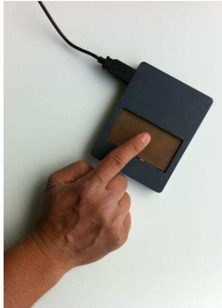
Figure 1-7: The optimized Stimtac version connected by a USB connection
