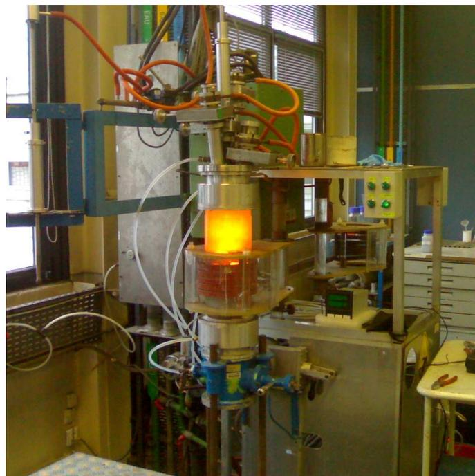
Photo of the 1 kg induction furnace during the metallic charge melting (yellow to orange light)
