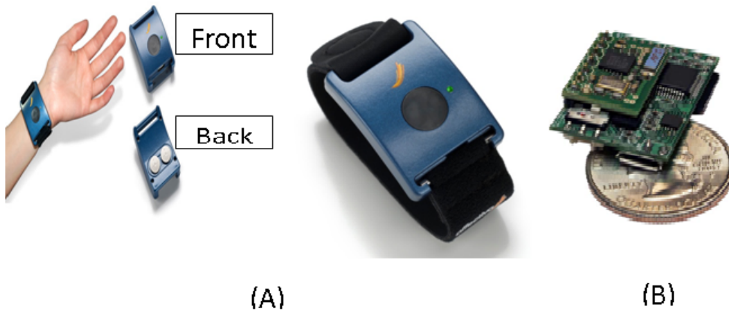
Figure 3.9: (A) The used EDA sensor (Q sensor): composed of a wristband and a pod where are inserted electrodes. (B) The Q sensor electronic module. (Source: www.Affectiva.com )
