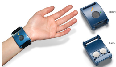
Figure 4.1: The used electrodermal activity sensor. It is composed of a wristband and a pod where are inserted electrodes (credit: Affectiva)
