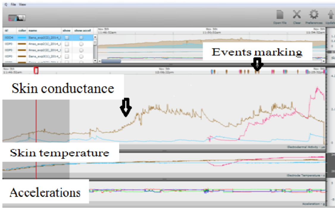
Figure 3.10: The EDA sensor dedicated software: It offers to the user the ability to visualize different sensor's recorded signals and marking special events
