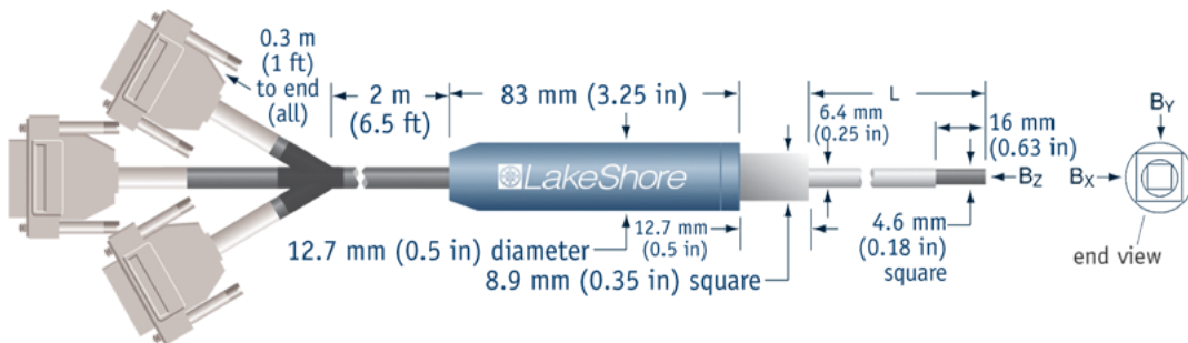
Figure 9.2 – Scheme of the HSE-1 tri-axis probe connectable to LakeShore Model 460 3-channels Gaussmeter (see Figure 9.3d)
