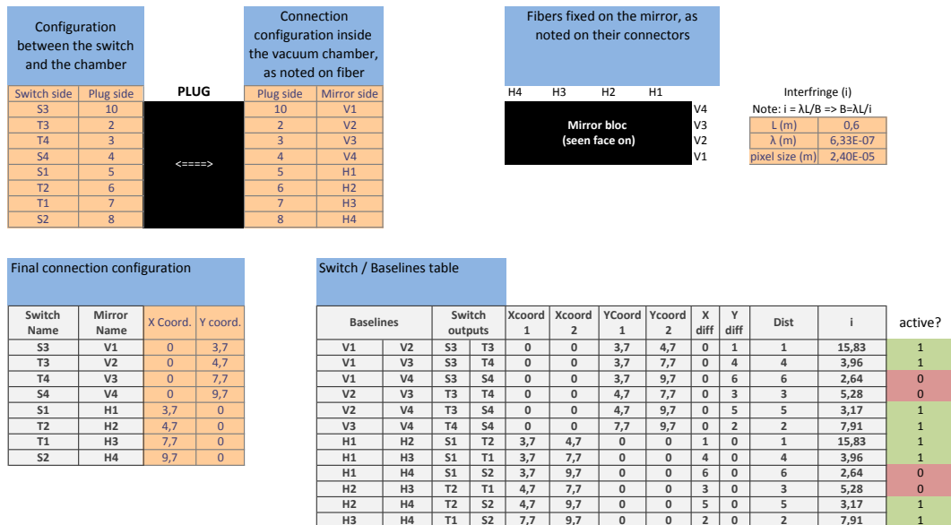
Figure E.6: Metrology configuration spreadsheet. It summarizes all the practical information needed about the current metrology configuration: how the connectors/fibers are paired between the switch and the vacuum plug, after the vacuum plug inside the vacuum chamber, what are the final baselines interfringe distances and what are the corresponding switch commands.
