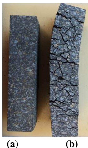
Figure II-23: MgO-C sample with an antioxidant Al before (a) and after (b) hydration
