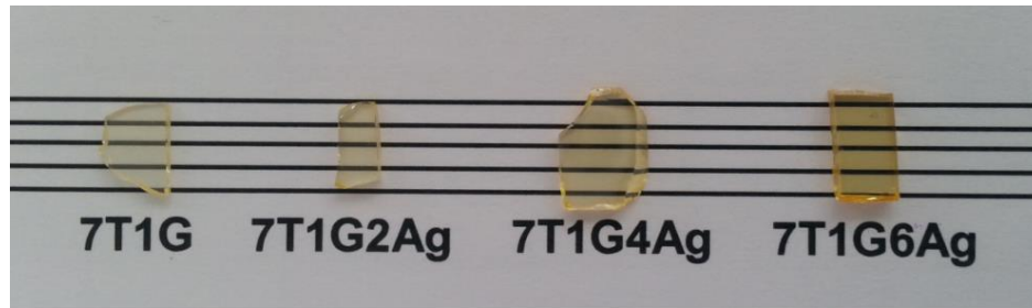
Figure 3.1: Elaborated (100-x) [70TeO 2 – 10GeO 2 – 10Nb 2 O 5 – 10K 2 O] – xAg 2 O (mol%) glass samples.
