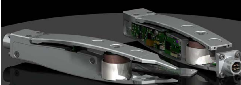
Figure 4.5: The haptic tweezers of the project NeuroArm for robotic surgery [Rizun 2006b].
