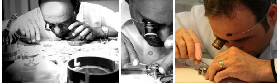
Figure 4.10: The third typical gesture to use tweezers in watchmaking process.
