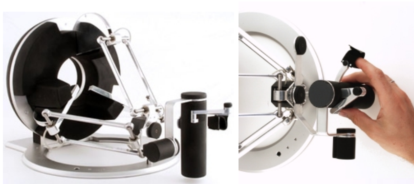
Figure 1.25: Haptic interface Omega 7 by Force Dimension [ForceDimension 2016].
