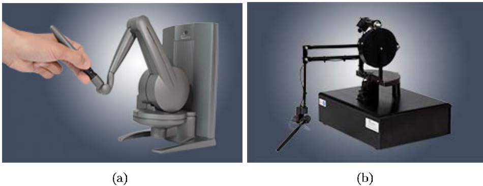
Figure 1.23: (a) PHANToM Desktop; (b) PHANToM Premium.
