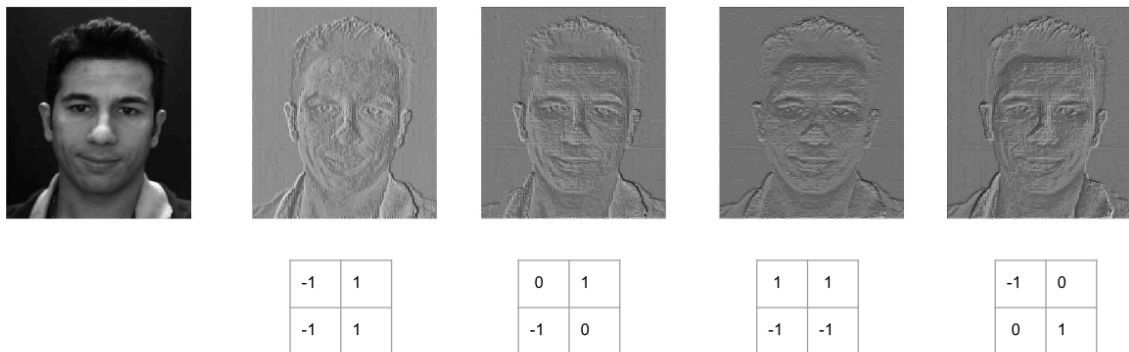
Fig. 3.1 Convolution of an image by four oriented gradient filters
