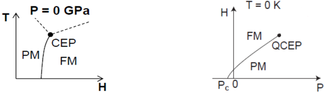
(a) ( T, H ) phase diagram of UCoAl at P = 0 . The 1 st order line ends at CEP(11K, \sim 1\text{T} ).
