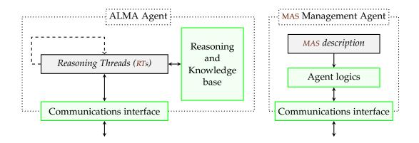
Figure 19: Defining an ALMA MAS, with normal agent architecture to the left and the MAS Management Agent (which includes the *yellow pages* service) to the right. Black rectangles represent the components provided by the programmer (RTs and the MAS description), with the rest (green) being provided by the platform. The dashed line represents the execution flow, while full lines are for information exchanges (messages, belief reads, rule writes).
