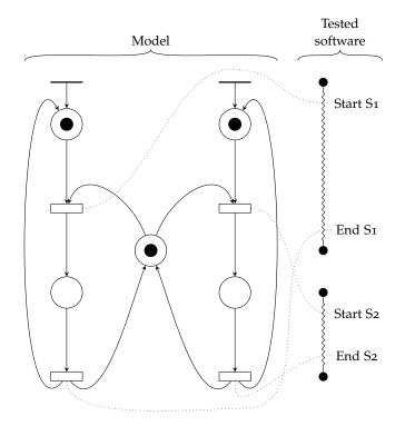
Figure 3: Petri net with corresponding observed code
