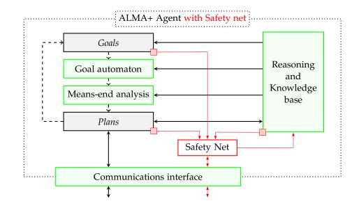
Figure 33: The architecture of an ALMA+ agent with safety net. Black rectangles represent the components provided by the programmer (goals and plans), the safety net mechanisms are represented in red and the rest (green) are provided by the platform. Dashed lines represent the execution flow, while full lines are for information exchanges (messages, belief reads, rule writes).
