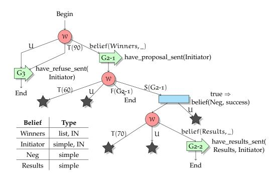
Figure 95: Plan P<sub>MCi2-1</sub> "worker part". Setting the "Neg" belief to true signals to the initiator part that it can continue its CFW, while adding a contradiction to the desirable belief causes the initiator part to stop.
