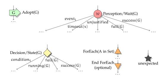
Figure 27: Proposed new nodes: *adopt* (extends action node), *wait* with new condition on goal end, a *decision* node for the outcome of a goal, *for each* nodes and finally an unexpected error node symbolising a case deemed impossible by the programmer, or in which the preferred reaction is given by our recovery mechanism. As exemplified in Fig. 28, the *End ForEach* is needed only if the plan does not finish with the *ForEach* block.
