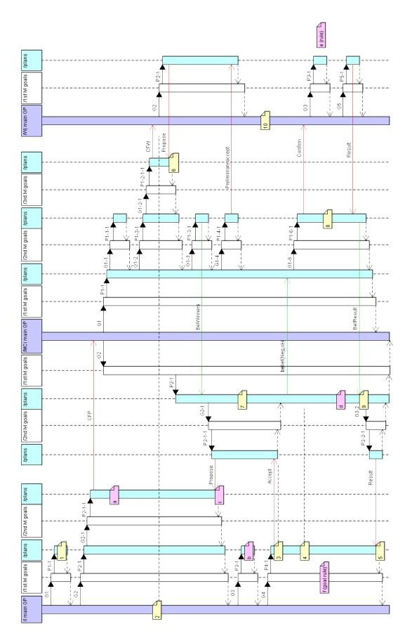
Figure 47: Sequence diagram for a successful CNP+ negotiation (the Initiator agent ends up with a result). Pink tags with letters correspond to the error cases from Sec. 5.4.1 and the yellow tags with numbers to the ones in Sec. 5.4.2.
