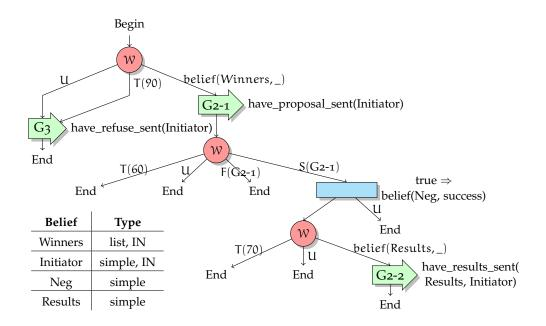
Figure 41: Plan  $P_{MCi2-1}$  "worker part". Setting the "Neg" belief to true signals to the initiator part that it can continue its CFW, while adding a contradiction to the desirable belief causes the initiator part to stop. This plan is very similar to the Worker agent's main goal plan.
