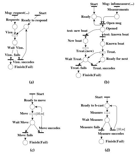
Figure 58: Petri net representations of the *GP*<sub>2</sub> (a), *GP*<sub>3</sub> (b), *GP*<sub>4</sub> (c) and *GP*<sub>5</sub> (d) goal plans. Goal adoptions are represented as hollow transitions.
