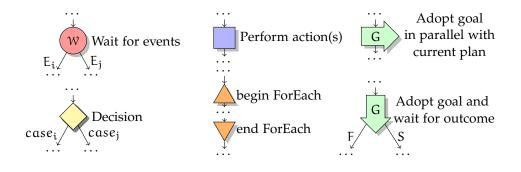
Figure 61: Flowchart nodes for efficiently describing the plans of goal-driven agents
