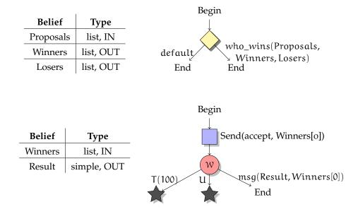
Figure 85: Plans  $P_{I3-1}$  - "get proposals sorted" and  $P_{I4-1}$  - "have work done". Plan  $P_{I3-1}$  simply uses an external method to sort according so some criteria and produce the two lists: Winners and Losers. The goal will fail if the Winner list is empty. Plan  $P_{I4-1}$  sends "accept" message to the **single** winner and waits for the reply.
