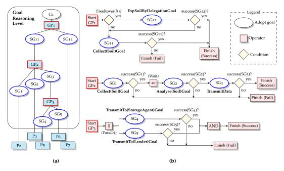
Figure 53: A multiple level goal plan for the Mars rover scenario from Fig. 49, with (a) the resulting goal-plan hierarchy (as used in Sec. 5.2 and similar to a GPT) representation and (b) the corresponding goal plans. Note the separation in (a) between the action plans, i.e. P2, P3, P5, P6 and P7, and the goal reasoning level comprising the goals and the three goal plans, i.e. GP1, GP2 and GP3.
