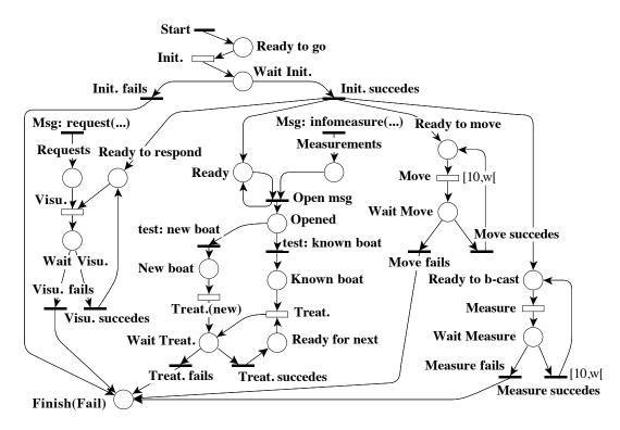
Figure 55: Petri net representation of the goal plan for the aircraft agent with goal adoptions represented as hollow transitions. The *Treat*. (for "treatment") goal is adopted in two different contexts in order to insure that messages from each boat are treated sequentially, but in parallel with the other boats. Multiple instances of the goal with different beliefs are thus created.
