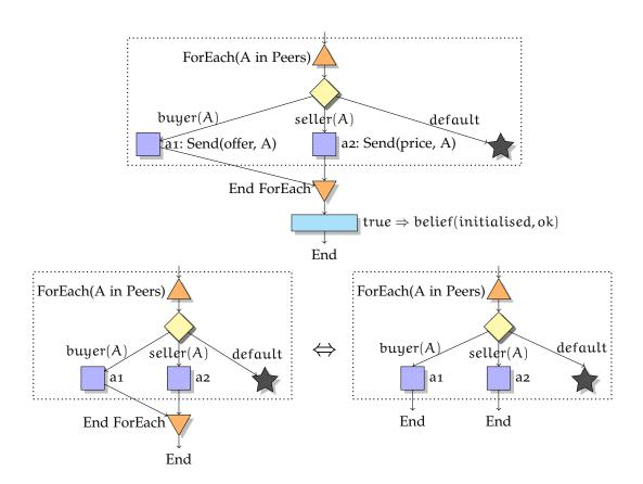
Figure 28: Examples for the use of the *ForEach* node. Note how at the end of a plan the *End ForEach* node is optional. Also, note that the *unexpected* node is a terminal node (just as an *End* node). The plan sections in the dotted rectangles are identical between them.
