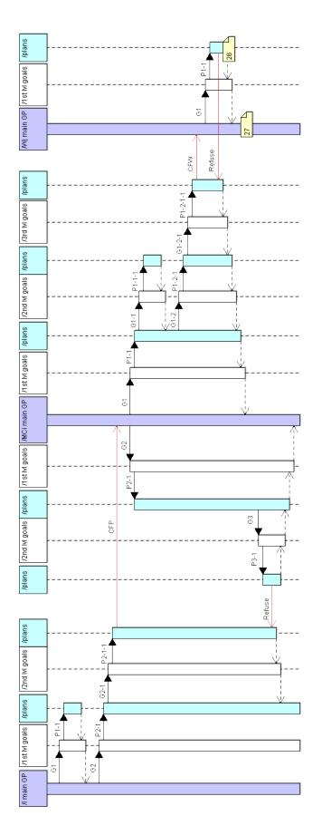
Figure 104: Sequence diagram for a successful CNP+ negotiation (the Initiator agent ends up with a result). Yellow tags correspond to error cases from Table 20.
