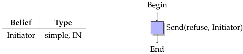
Figure 88: Plan P_{MCi3-1} “have refuse sent” that refuses the CFP with a message to the Initiator
