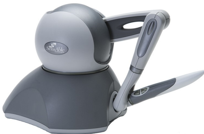
FIGURE 4.9 – Bras haptique Phantom Omni.
