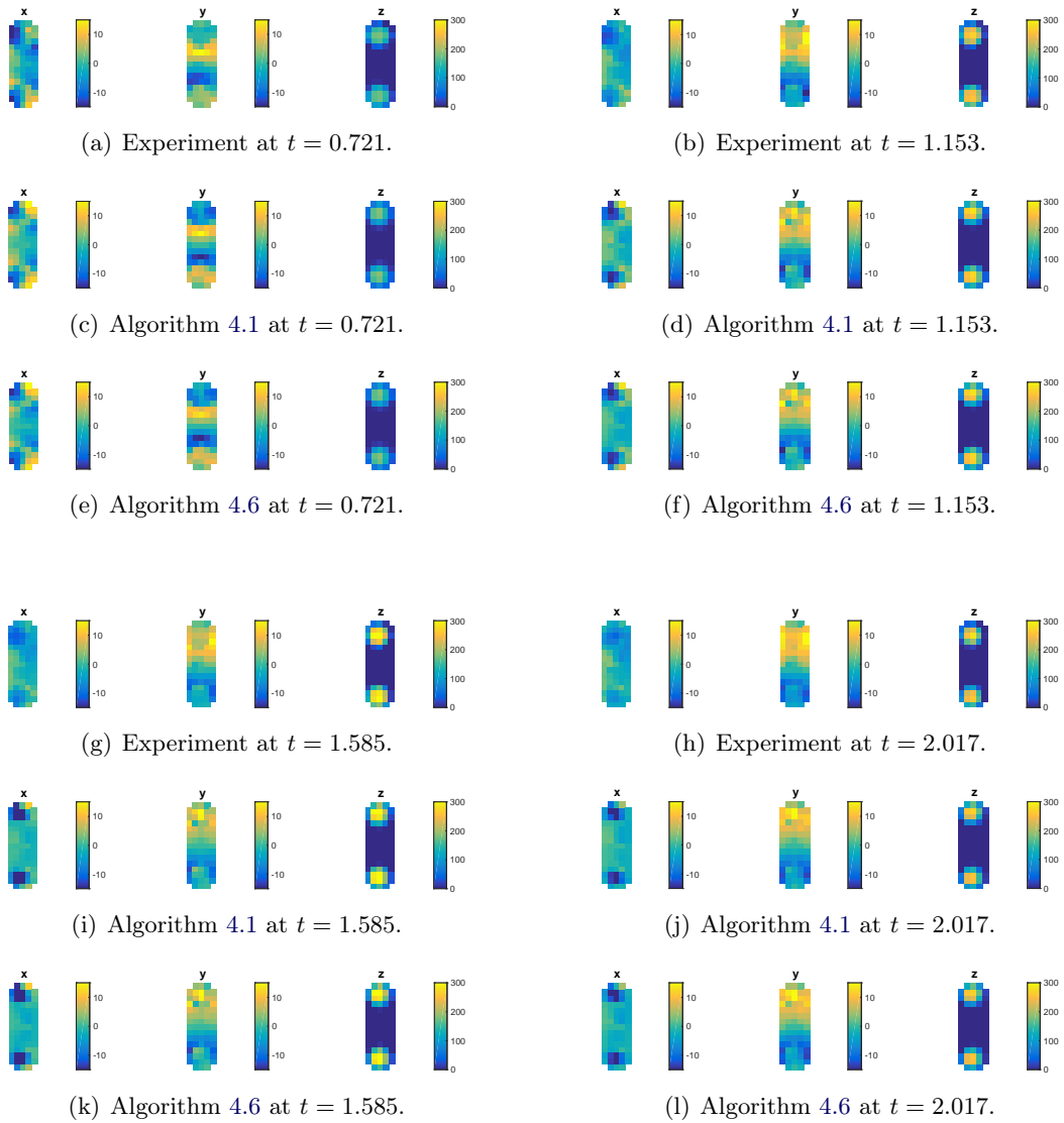
Figure A.3: Fluid velocity components in Phase II. Comparison of the experimental data with the predictions obtained with Algorithms 4.1 and 4.6. Plane z = 3.5 . Units are mm\ s^{-1} .
