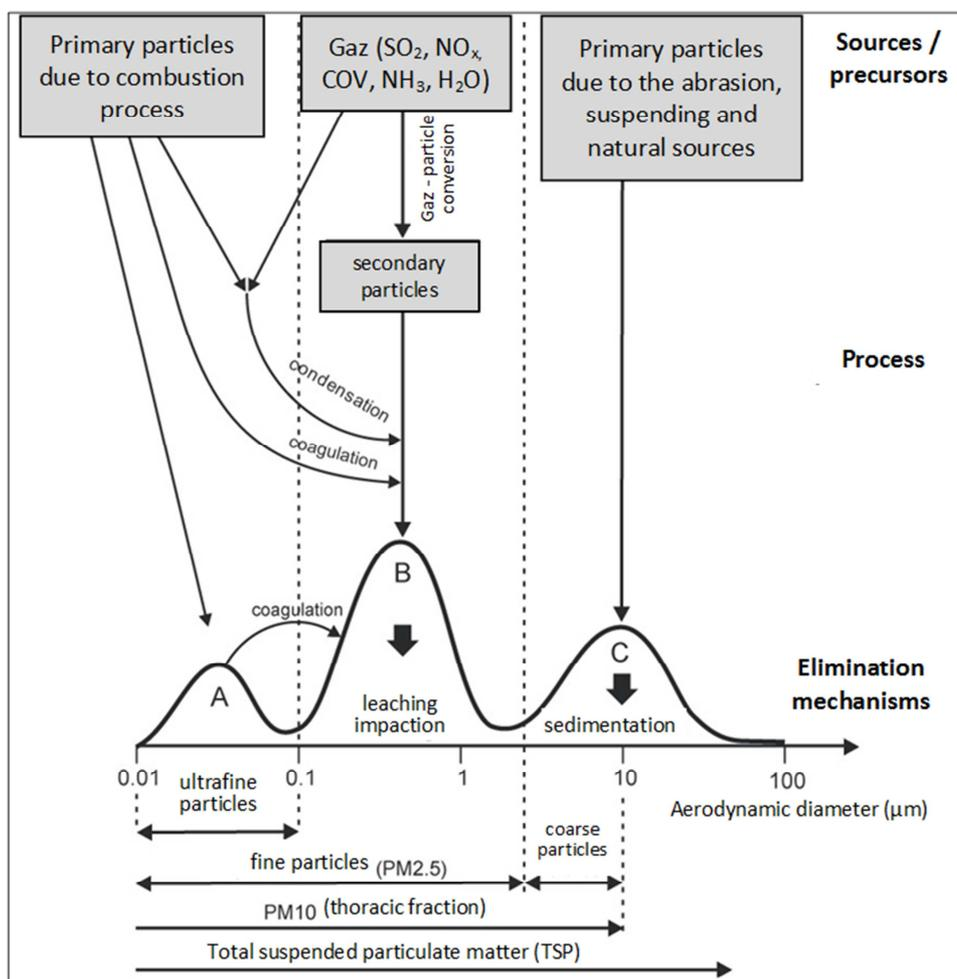
Fig. 1. Simplified size distribution of atmospheric aerosol particles and important process. A = ultrafine particles, B = accumulation mode, C = Coarse particles. Away from sources, mode B predominates. Source: DETEC (2011)
