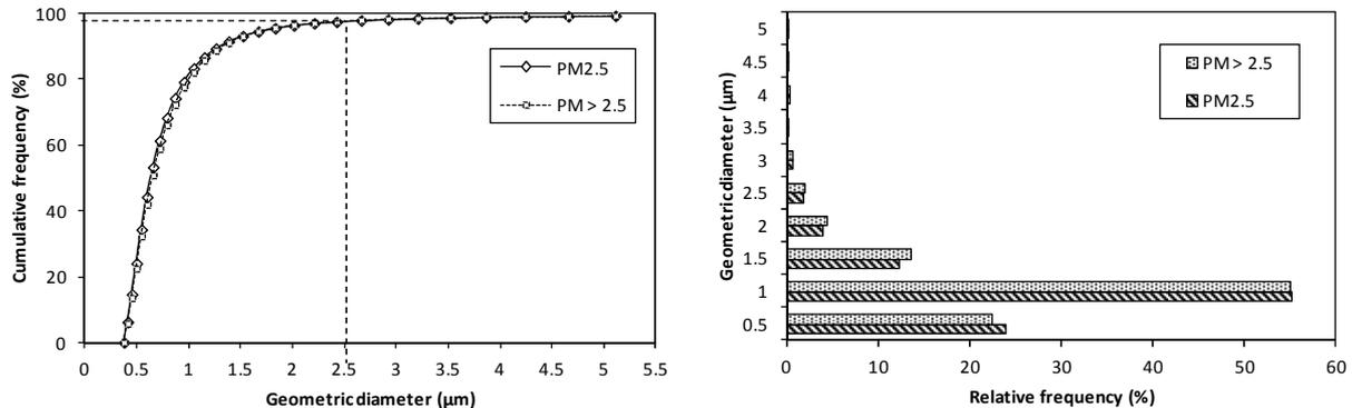
Fig. 3. Size distribution by cumulative frequency (%) and relative frequency (%) of PM<sub>2.5</sub> and PM<sub>>2.5</sub> collected in an urban site, Cotonou.
