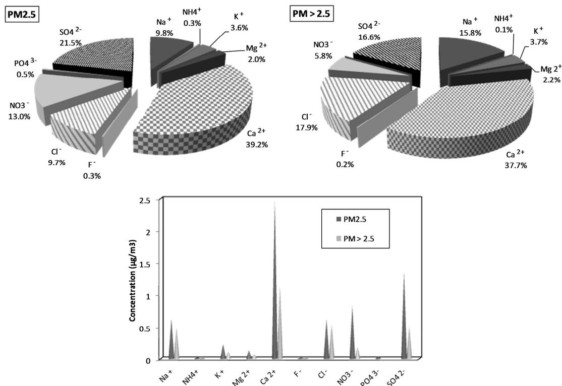
Fig. 4. Ionic species concentrations of the two aerosols collected are in species mass per air volume pumped and in percentage. The concentration of PO<sub>4</sub><sup>3-</sup> was under of quantification limit in PM<sub>>2.5</sub>.
