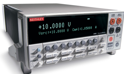
Figure II.7 – Photo d'un Keithley 2400 source-meter.
