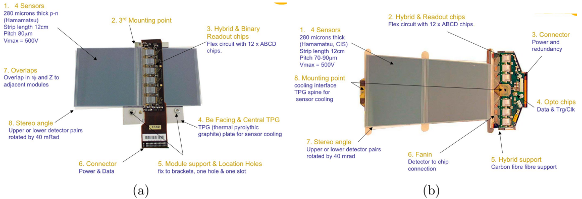
Figure 2.12: (a) SCT barrel module and (b) SCT end-cap module.
