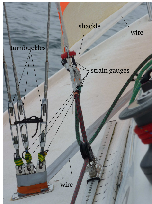
Figure 2.13 – Picture taken during experiments showing load sensors on the shackle of the jib sheet, and on the shrouds on portside.
