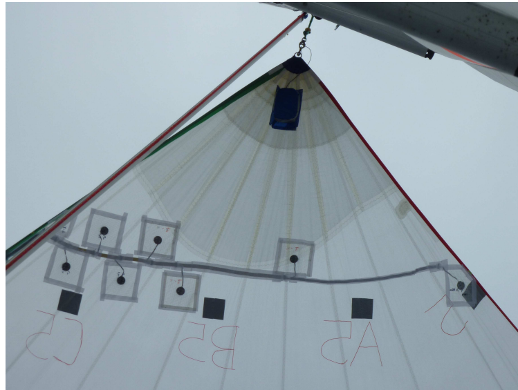
Figure 2.19 – Top of the spinnaker where the 7/8 stripe and its 8 pressure taps are visualised. The squares around them corresponds to the contour of light sail cloth patches.
