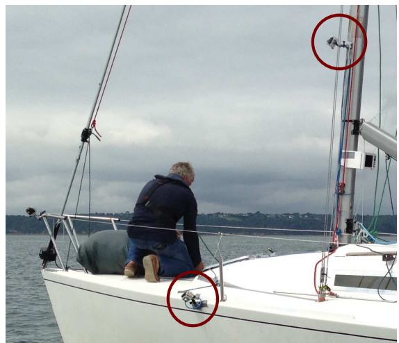
(f) Position of camera GP2Y on the deck-hull connection on portside and camera GP2W on the mast.
