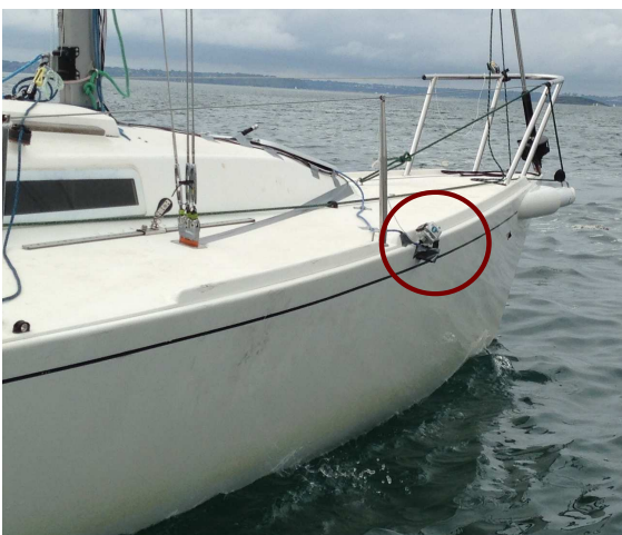
(e) Position of camera GP2G on the deck-hull connection on starboard side.
