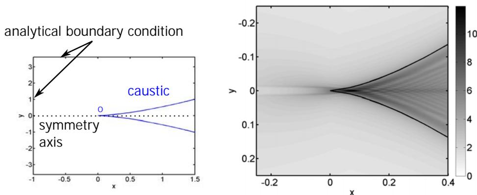
**Figure 3.2.** – Left : schematic diagram of the domain of calculation used for the caustic cusp geometry.  $O$  is the geometrical caustic point, at the origin. Right : maximum particle velocity determined by the numerical solution for a focused N-wave for the case  $N_\tau = 70001$ . The geometrical caustic cusp is shown as a line. The solution is zoomed around the caustic cusp.
