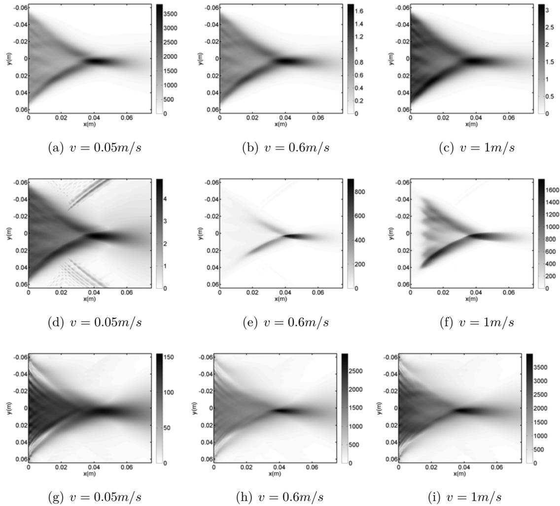
**Figure 3.9.** – Maximum of energy (top), acceleration (middle) and shear stress  $\sigma_{31}$  (bottom) on the calculation domain for initial amplitudes of  $0.05m/s$  (left),  $0.6m/s$  (middle) and  $1m/s$  (right). These values correspond to shock formation distances that are, respectively, well past the focus, near the focus, and well before the focus.
