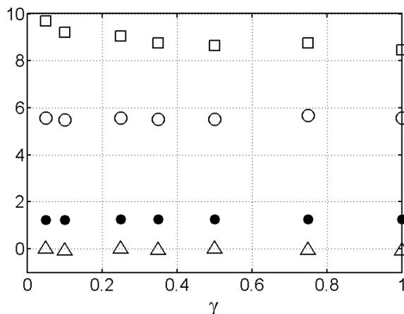
**Figure 3.5.** – Values of self-similar variables  $\bar{x}$  (circle),  $\bar{y}$  (triangle),  $\bar{v}$  (disk),  $-\bar{t}$  (square) of the point of maximum amplitude for different values of  $\gamma$ . In the ideal case each value would follow a horizontal line.
