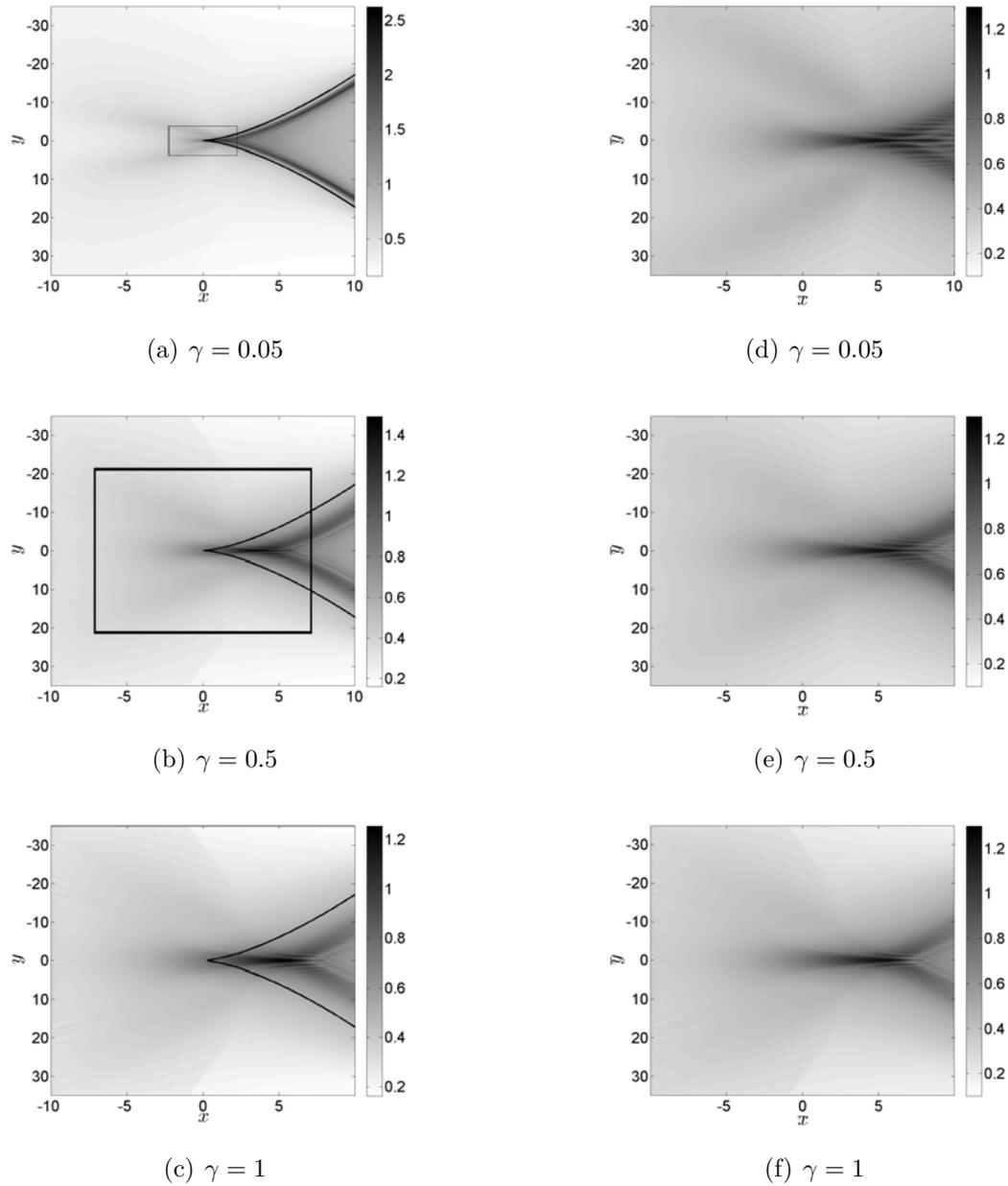
**Figure 3.4.** – Velocity field for different values of  $\gamma$  for the self-similar case of a focused step shock with boundary condition given by Eq.(3.26). Left column : direct simulations calculated on a fixed domain. The solid line is the geometrical cusp caustic. Right column : the same simulations rescaled by the self-similar variables. The rectangles on the left column show the rescaled region in the right column.
