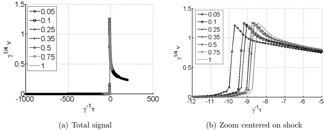
**Figure 3.6.** – Velocity as a function of retarded time (self-similar variables) at the point of maximum amplitude for  $\gamma$  varying from 0.05 to 1. Left : full time signal. Right : zoom centered on the shock.
