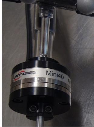
Figure 4-15: Force and torque sensor
