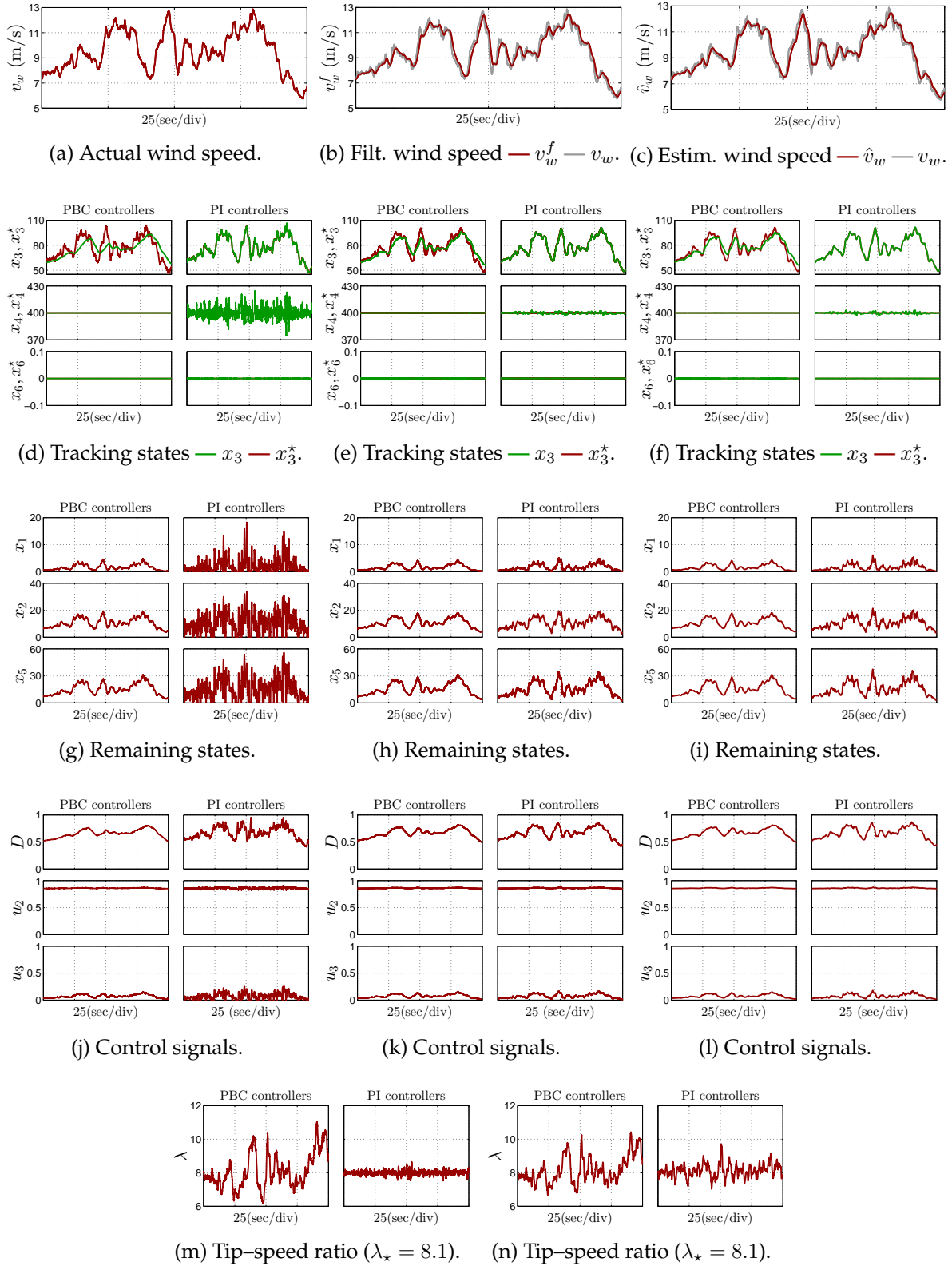
Figure 5.12: Simulation results. The left, middle and right columns presents the comparative evaluation utilizing the actual, filtered and estimated wind speed, respectively. Recall x := \text{col}(i_d, i_q, r\omega_m, v_{dc}, I_d, I_q) , hence the units for the various plots are: x_1 (A), x_2 (A), x_3 (m/s), x_4 (V), x_5 (A), x_6 (A). Control signals are unitless and because of their physical interpretation they must be contained within 0 and 1.
