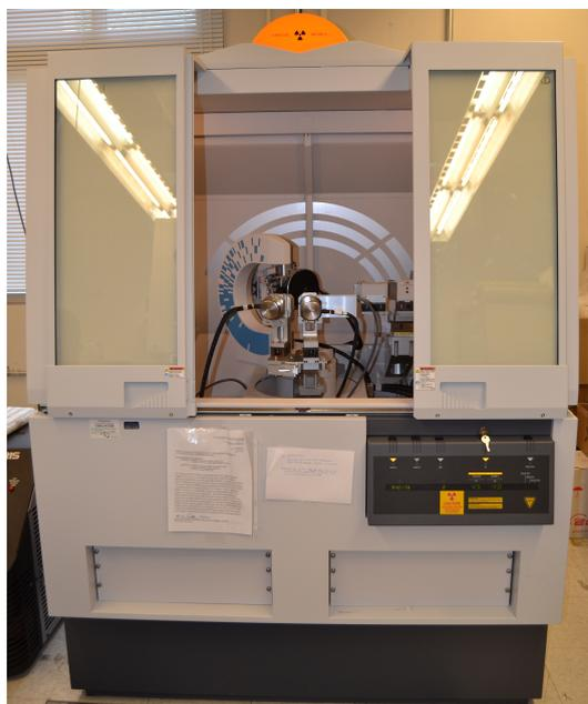
Figure 5.21: Picture of the X'Pert<sup>3</sup> PRO MRD diffractometer from PANalytical.
