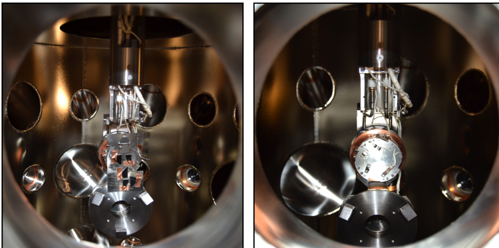
Figure 4.9: Pictures of the sample holders used at room temperature (left) and at low temperature (right).
