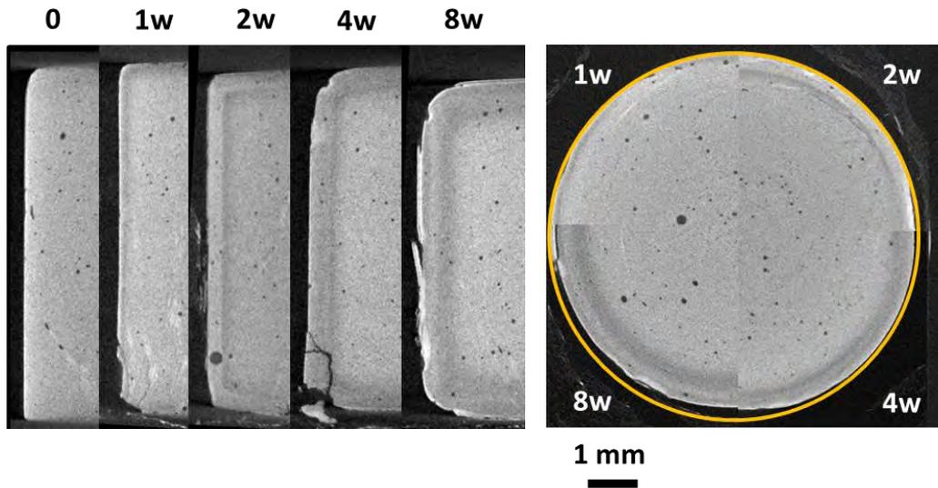
Figure 19: Frontal (left) and transverse (right)  $\mu$ -CT images of  $\beta$ -TCP samples after different times of immersion in TRISd (resolution of  $10 \mu\text{m}/\text{voxel}$ ). The circle in yellow (transverse section) represents the circumference of the sample at  $t_0$
