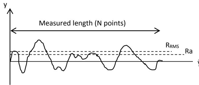
Figure 10: Two parameters of roughness ( $R_a$  and  $R_{RMS}$ )
