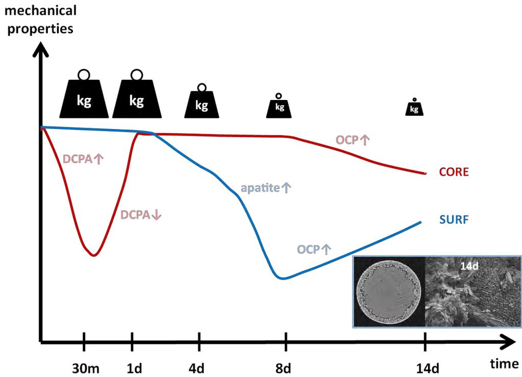
Figure 47: Schematic representation of the main changes observed during immersion of DCPD samples in TRISd. The weights for scales represent the changes of the sample mass
