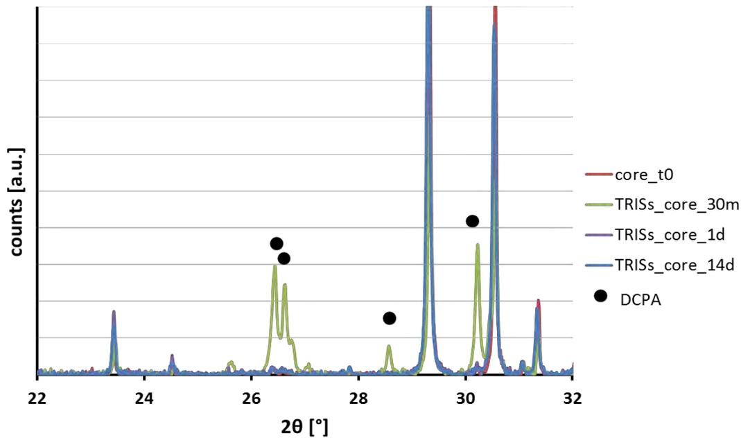
Figure 19: XRD patterns of DCPD samples in the core at time 0, after 30minutes, 1 and 14 days in TRISs. For clarity purposes the y-axis is showed till half the height of the highest peak and non-indexed peaks correspond to DCPD phase.
