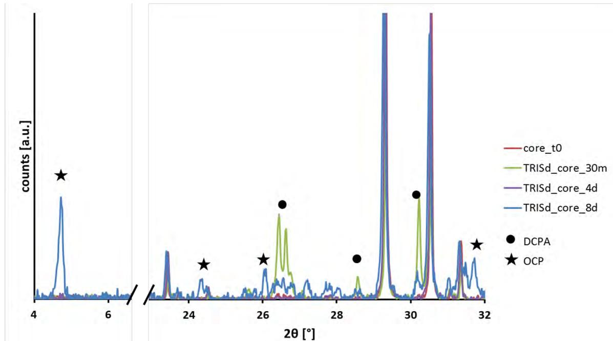
Figure 20: XRD patterns of DCPD samples in the core at time 0, after 30 minutes, 4 and 8 days in TRISd; For clarity purposes the y-axis is showed till half the height of the highest peak and non-indexed peaks correspond to DCPD phase.
