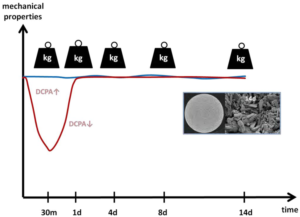
Figure 48: Schematic representation of the main changes observed during immersion of DCPD samples in TRISs. The weights for scales represent the changes of the sample mass
