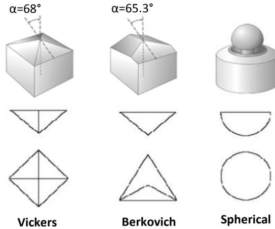
Figure 19: Main geometries of tips used for indentation and the correspondent traces left on samples (cross and horizontal section) [3]
