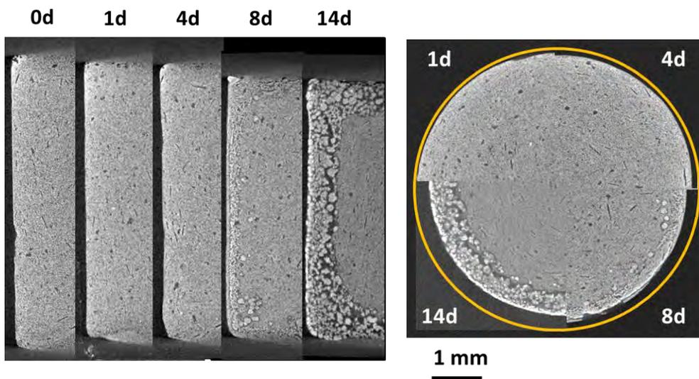
Figure 28: Frontal (left) and transverse (right)  $\mu$ -CT images of DCPD after different times of immersion in TRISd (resolution of  $10 \mu\text{m}/\text{voxel}$ ). The circle in yellow (transverse section) represents the circumference of the sample at  $t_0$
