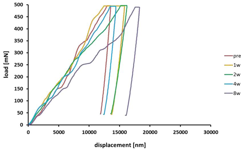
Figure 30: Representative load-displacement curves obtained at the surface of  $\beta$ -TCP samples after immersion in PBSd
