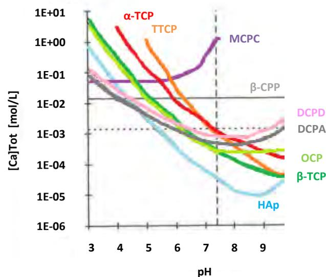
Figure 10: Isotherm curves of solubility of CaP (in water, 25°C). From top to bottom: MCPM,  $\beta$ -CPP (flat line),  $\alpha$ -TCP, TTCP, DCPD, DCPA, OCP,  $\beta$ -TCP, HAp. The solubility is expressed as the total concentration of calcium ions dissolved in solution. Dotted line: Ca ions concentration in human serum/blood. Dashed line: pH of human serum [6, 45, 82, 83]
