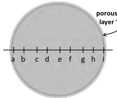
Figure 42: Scheme of the section of a degraded sample, after 1 weeks of immersion TRISd. The letters correspond to the points where indentations were performed. The darker ring close to the surface represents the porous layer observed by  $\mu$ -CT
