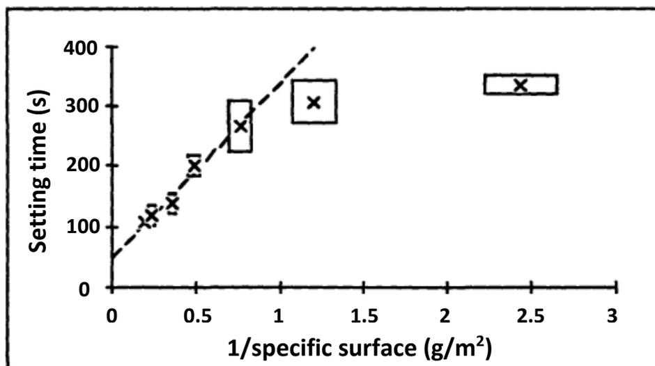
Figure 7: Setting time vs inverse ratio of the specific surface of  $\beta$ -TCP powder (squares = 90% confidence level).
