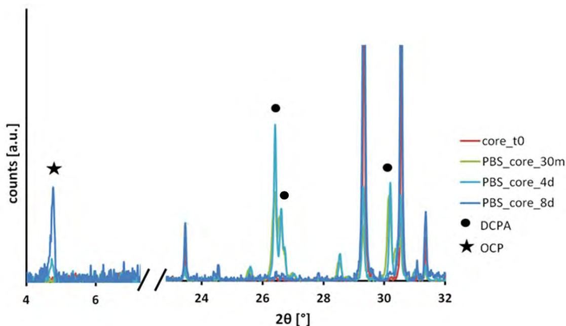
Figure 18: XRD patterns of DCPD samples in the core at time 0, after 30 minutes, 4 and 8 days in PBSd. For clarity purposes the y-axis is showed till half the height of the highest peak and non-indexed peaks correspond to DCPD phase.
