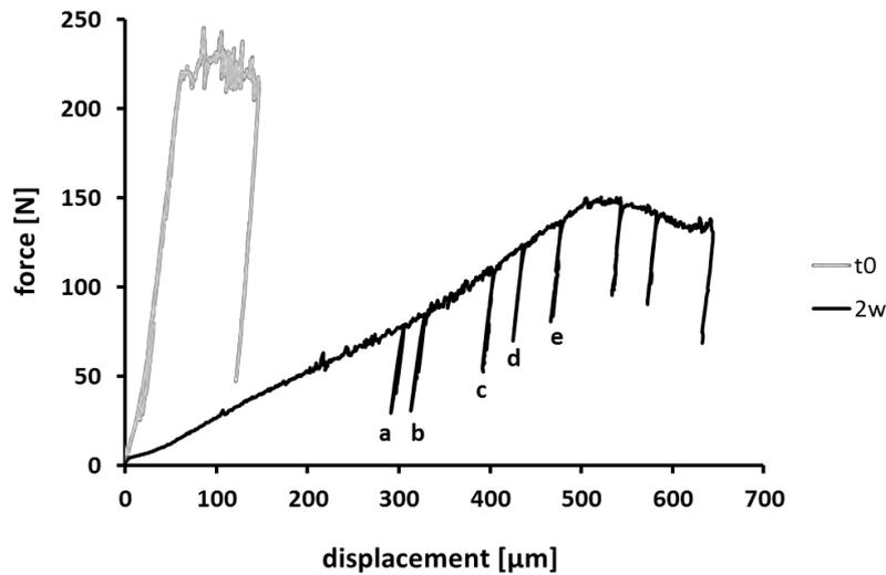
Figure 44: Representative compressive force-displacement curves before (in grey) and after two weeks (in black) immersion in TRISd. Loading/unloading cycles (a, b, c, d, e...) can be noted on the curve after immersion.
