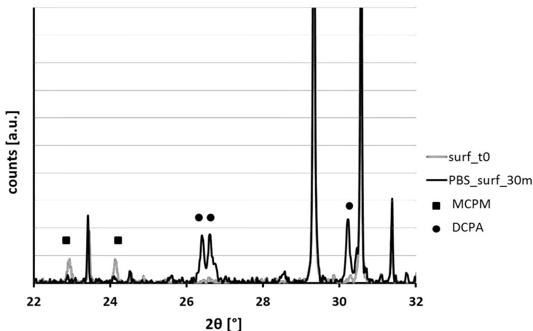
Figure 14: XRD patterns of the surface of DCPD samples at time 0 and after 30 minutes in PBSd. Peaks, which are not marked, correspond to the DCPD phase. For clarity purposes the y-axis is showed till half the height of the highest peak
