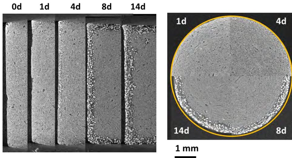
Figure 24: Frontal (left) and transverse (right)  $\mu$ -CT images of DCPD samples after different times of immersion in PBSd (resolution of  $10 \mu\text{m}/\text{voxel}$ ). The circle in yellow (transverse section) represents the circumference of the sample at  $t_0$
