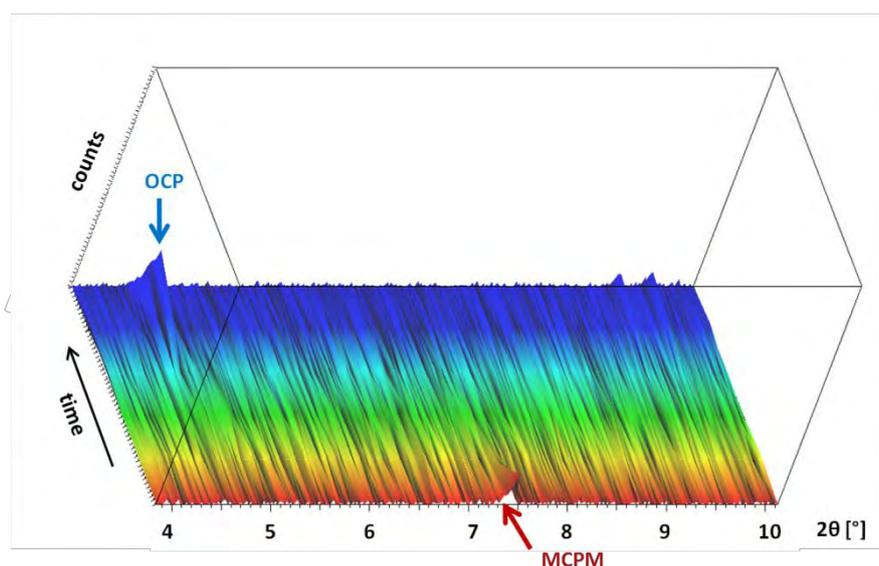
Figure A.b.2: Evolution during time (0-14d) of phases at the surface of DCPD samples after immersion in PBS.
