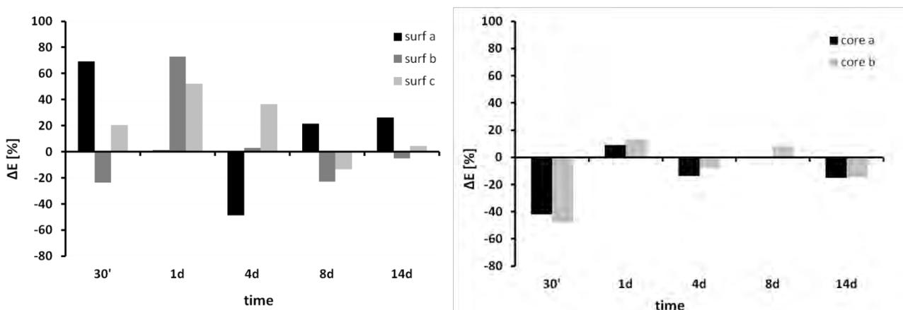
Figure A.b.18: Variation of Young's Modulus of DCPD samples at the surface (left) and in the core (right) after different immersion times in TRISs. Average values at  $t_0$ :  $H_{surface}=9.2MPa$ ,  $E_{surface}=1101MPa$ ,  $H_{core}=6.1MPa$ ,  $E_{core}=882MPa$
