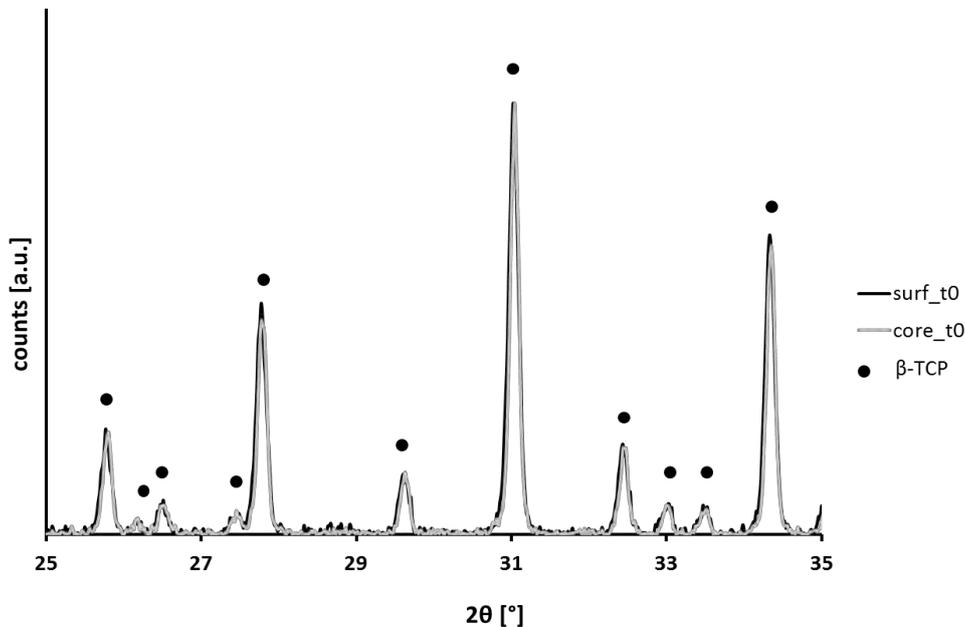
Figure 1: XRD pattern of  $\beta$ -TCP samples at the surface (in black) and in the core (in grey) before immersion
