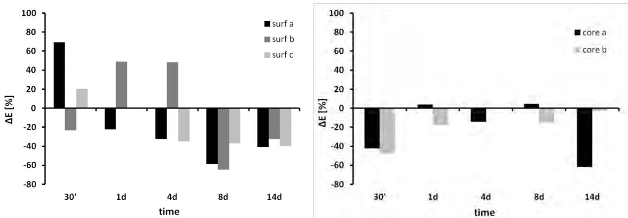
Figure A.b.20: Variation of Young's Modulus of DCPD samples at the surface (left) and in the core (right) after different immersion times in TRISd. Average values at  $t_0$ :  $H_{\text{surface}}=9.2\text{MPa}$ ,  $E_{\text{surface}}=1101\text{MPa}$ ,  $H_{\text{core}}=6.1\text{MPa}$ ,  $E_{\text{core}}=882\text{MPa}$
