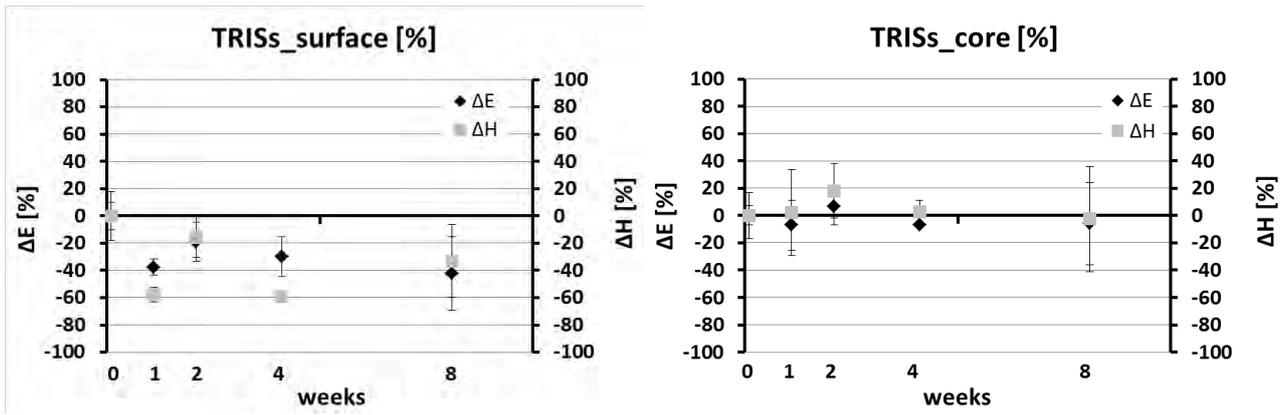
Figure 32: Variation of H and E at the surface (left) and in the core (right) of  $\beta$ -TCP samples after different immersion times in TRISs
