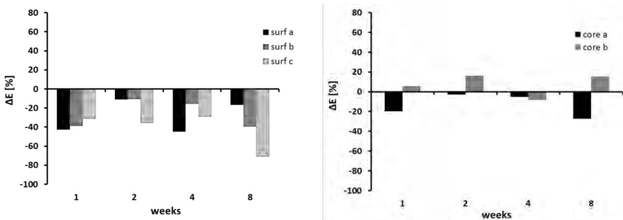
Figure A.c.8: Variation of Young's Modulus of  $\beta$ -TCP samples at the surface (left) and in the core (right) after different times of immersion in TRISs. Average values at  $t_0$ :  $H_{surface}=5.0MPa$ ,  $E_{surface}=788MPa$ ,  $H_{core}=3.8MPa$ ,  $E_{core}=986MPa$
