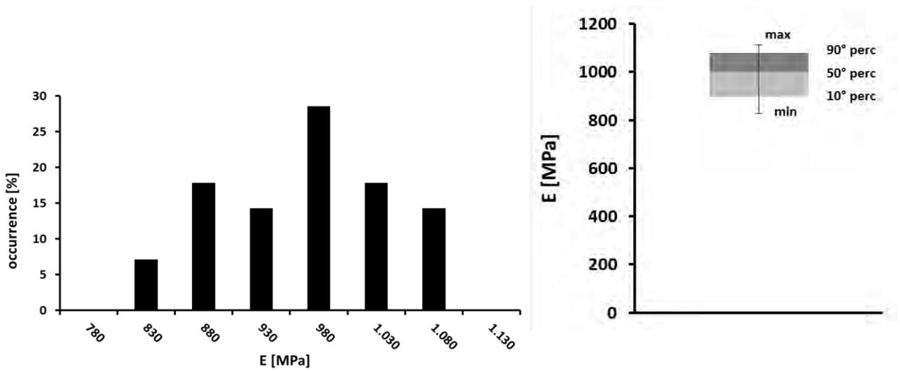
Figure 8: Distribution of values of Young's Modulus obtained in the core for all  $\beta$ -TCP samples at  $t_0$
