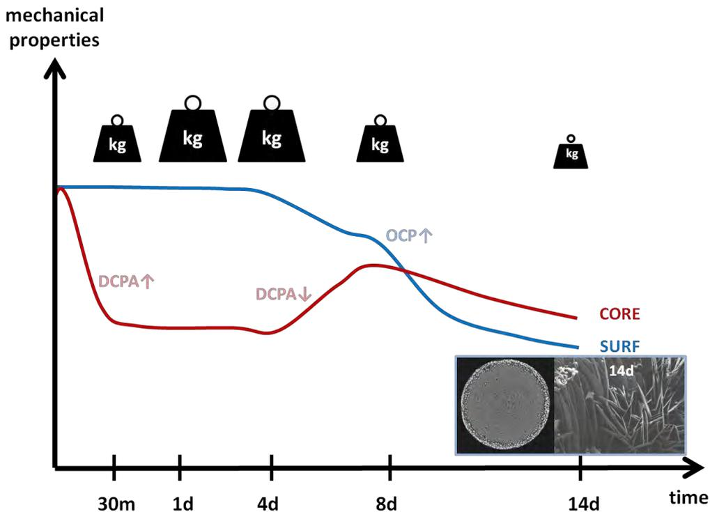
Figure 46: Schematic representation of the main changes observed during immersion of DCPD samples in PBS. The weights for scales represent the changes of the sample mass
