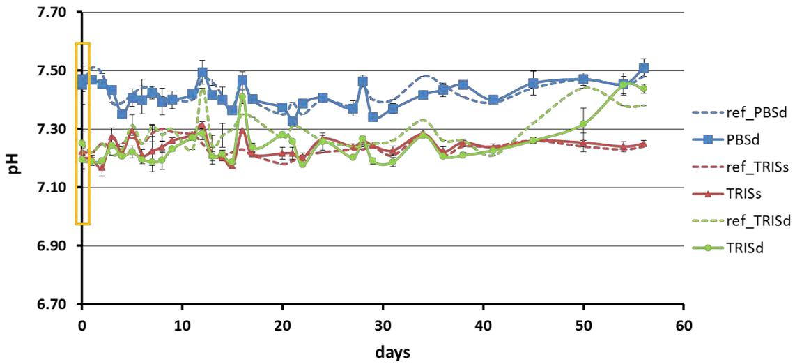
Figure 15: Evolution of pH of the solutions along the 8 weeks of test: solid lines for solutions containing samples and dotted lines for reference solutions (without samples).
