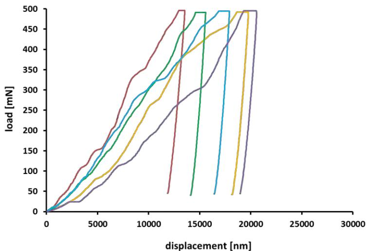
Figure 34: Representative load-displacement curves obtained in the core of  $\beta$ -TCP samples after immersion in TRISs
