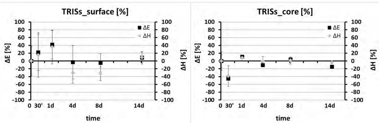
Figure 38: Variation of H and E at the surface (left) and in the core (right) after different times of immersion in TRISs
