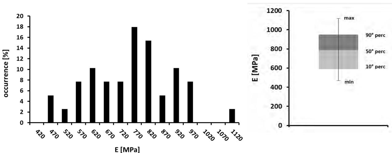
Figure 6: Distribution of values of Young's Modulus obtained at the surface for all  $\beta$ -TCP samples at  $t_0$
