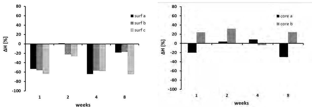
Figure A.c.7: Variation of hardness of  $\beta$ -TCP samples at the surface (left) and in the core (right) after different times of immersion in TRISs. Average values at  $t_0$ :  $H_{surface}=5.0MPa$ ,  $E_{surface}=788MPa$ ,  $H_{core}=3.8MPa$ ,  $E_{core}=986MPa$
