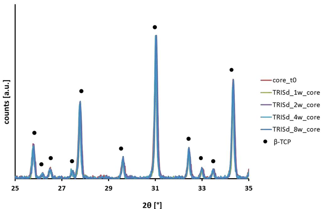
Figure A.c.3: XRD patterns of  $\beta$ -TCP samples in the core at time 0 and after 1-2-4-8 weeks in TRISd
