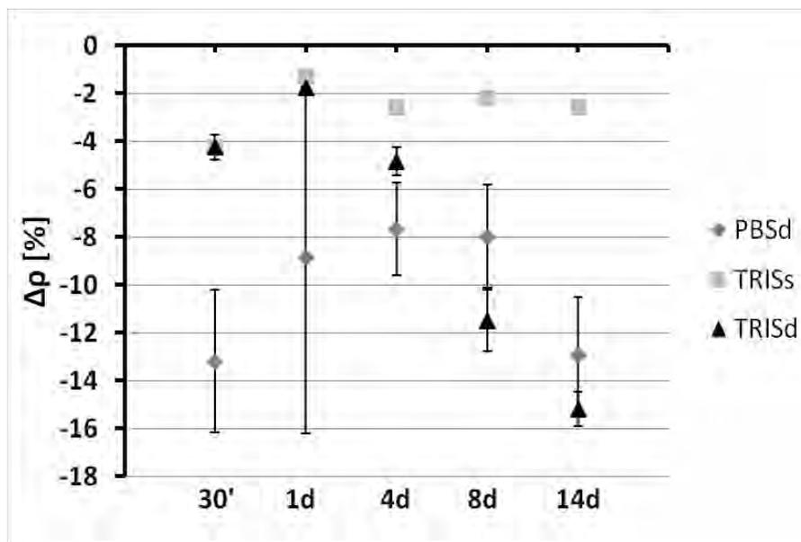
Figure 10: Percent variation of apparent density of samples after immersion (average density at  $t_0 = 0.91 \pm 0.01$  g/cm<sup>3</sup>),  $n=3$
