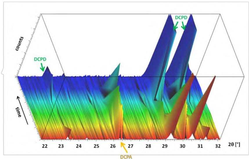
Figure A.b.5: Evolution during time (0-14d) of phases in the core of DCPD samples after immersion in PBS. Range  $2\theta = 22^\circ - 32^\circ$
