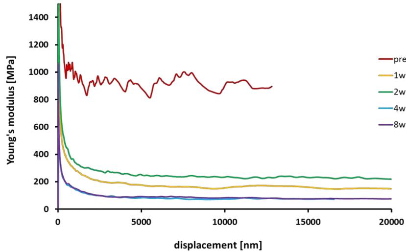
Figure 38: Representative Young's modulus-displacement curves obtained with the CSM method at the surface of  $\beta$ -TCP samples after immersion in TRISd
