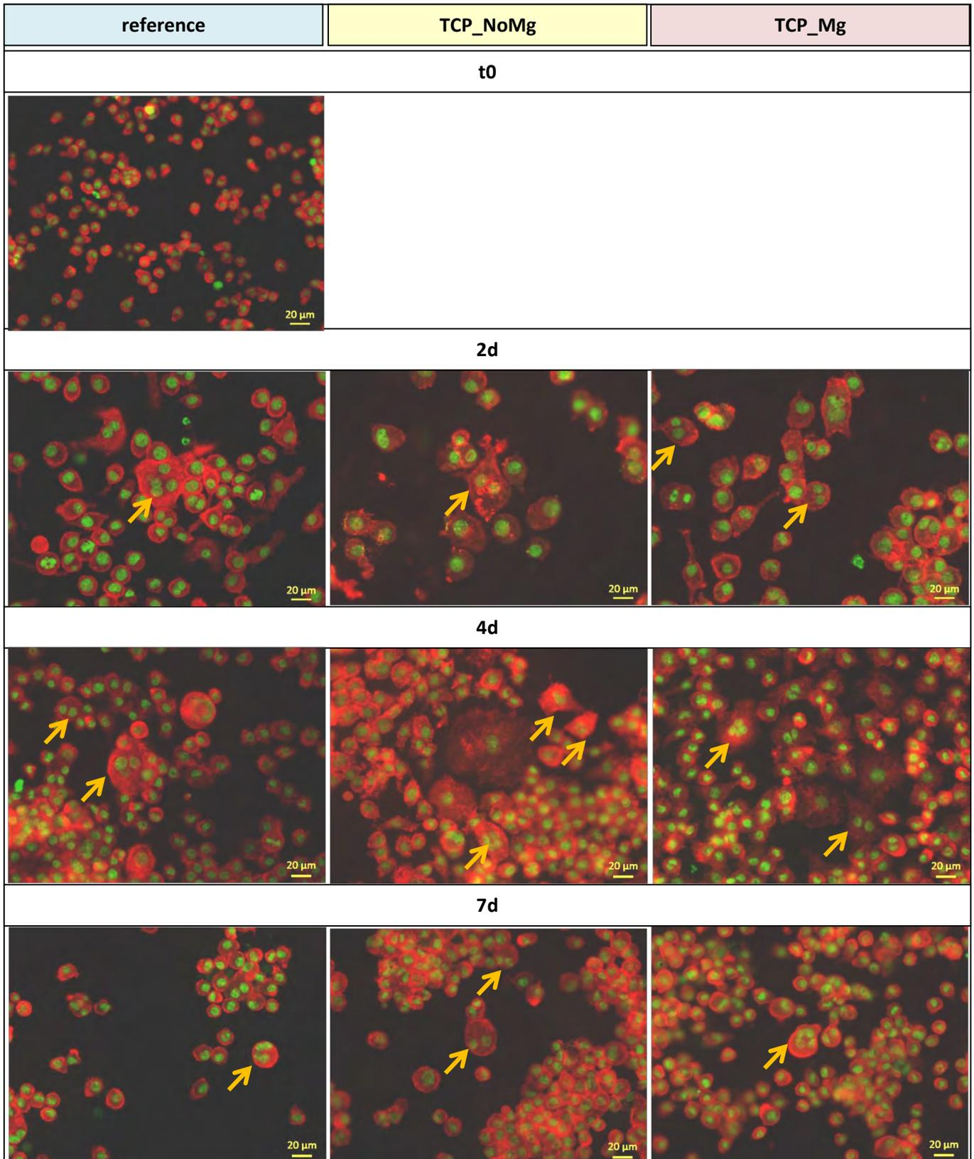
Figure 9: Fluorescence images of cells cultured on reference and  $\beta$ -TCP samples for different times. Actin filaments of the cytoskeleton appear in red, cell nuclei in bright green and arrows point out multinucleated cells.
