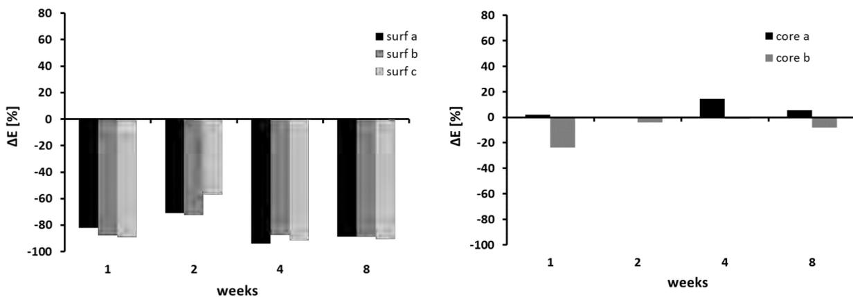
Figure A.c.10: Variation of Young's Modulus of  $\beta$ -TCP samples at the surface (left) and in the core (right) after different times of immersion in TRISd. Average values at  $t_0$ :  $H_{surface}=5.0MPa$ ,  $E_{surface}=788MPa$ ,  $H_{core}=3.8MPa$ ,  $E_{core}=986MPa$
