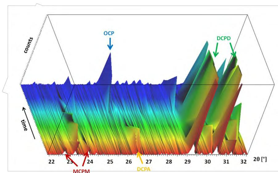
Figure A.b.1: Evolution during time (0-14d) of phases at the surface of DCPD samples after immersion in PBS.
