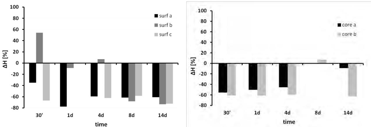
Figure A.b.15: Variation of hardness of DCPD samples at the surface (left) and in the core (right) after different immersion times in PBSd. Average values at  $t_0$ :  $H_{surface}=9.2MPa$ ,  $E_{surface}=1101MPa$ ,  $H_{core}=6.1MPa$ ,  $E_{core}=882MPa$
