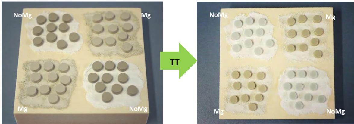
Figure 7: Production of dense  $\beta$ -TCP samples - samples before and after thermal treatment (TT). Specimens were placed on a layer of powder with the same chemical composition as the samples to hinder diffusion.
