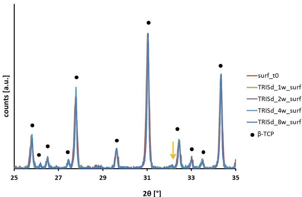
Figure 14: XRD patterns of  $\beta$ -TCP samples at the surface at time 0 and after 1-2-4-8 weeks in TRISd (arrow = peak at 32.1°)
