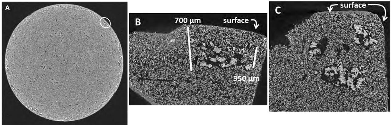
Figure 25: transverse  $\mu$ -CT image of DCPD after 4 days in PBSd (A) (resolution of  $10 \mu\text{m}/\text{voxel}$ ). Higher resolution images of the circled area in A (transverse B, frontal C), resolution of  $2 \mu\text{m}/\text{voxel}$
