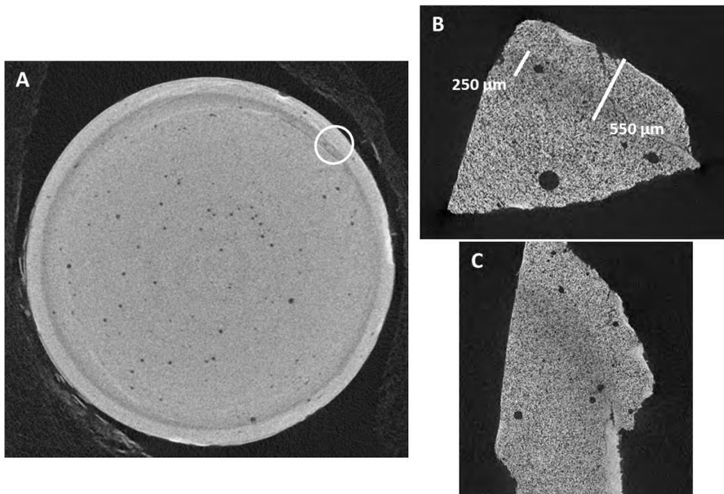
Figure 20: Transverse  $\mu$ -CT image of  $\beta$ -TCP samples after 2 weeks in TRISd (resolution of  $10 \mu\text{m}/\text{voxel}$ ) (A). Higher resolution images of the circled area in A (transverse B, frontal C,  $2 \mu\text{m}$  voxel size)
