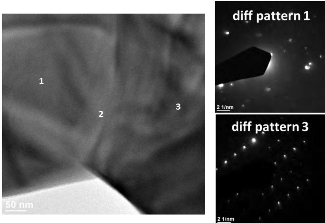
Figure 3: TEM image of TCP\_Mg (left) and diffraction patterns corresponding to zone 1 and 3 (right) (Images: L. Joly-Pottuz). Numbers correspond to areas where EDX analyses were performed
