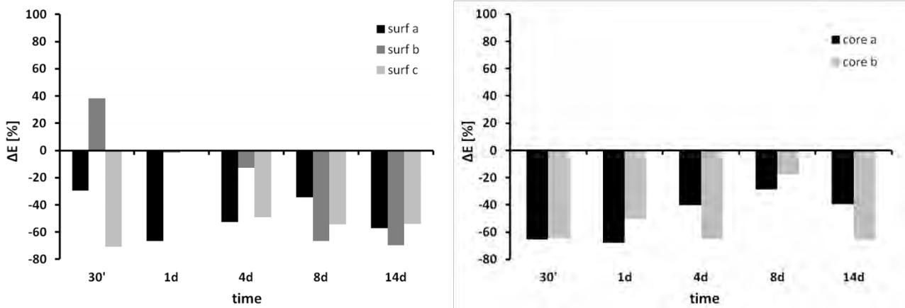
Figure A.b.16: Variation of Young's Modulus of DCPD samples at the surface (left) and in the core (right) after different immersion times in PBSd. Average values at  $t_0$ :  $H_{surface}=9.2MPa$ ,  $E_{surface}=1101MPa$ ,  $H_{core}=6.1MPa$ ,  $E_{core}=882MPa$
