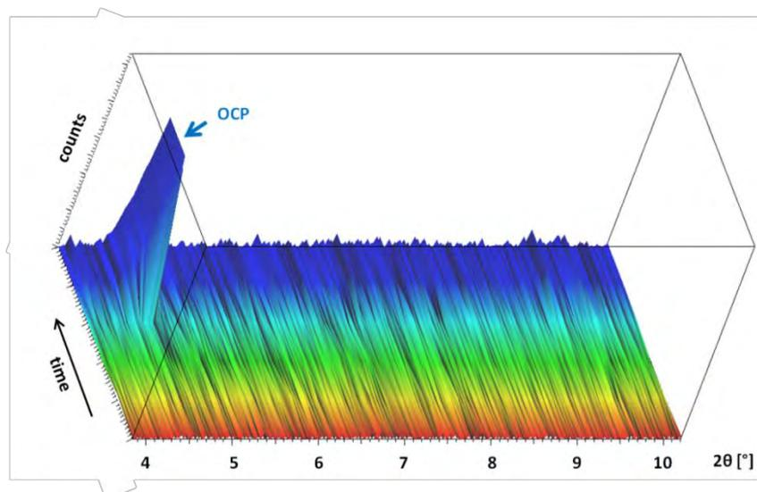
Figure A.b.8: Evolution during time (0-14d) of phases in the core of DCPD samples after immersion in TRISd. Range  $2\theta = 4^\circ - 10^\circ$
