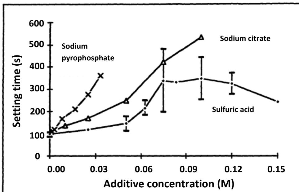
Figure 8: Effect of retardant concentration on setting time. Retardants:  $\text{Na}_4\text{P}_2\text{O}_7$ ,  $\text{C}_6\text{H}_5\text{O}_7\text{Na}_3$ ,  $\text{H}_2\text{SO}_4$  (only for sulfuric acid, bars = 90% confidence level). Cement composition: 1.5 g  $\beta$ -TCP, 1.2 ml solution 2M phosphoric acid and the retardant [59]
