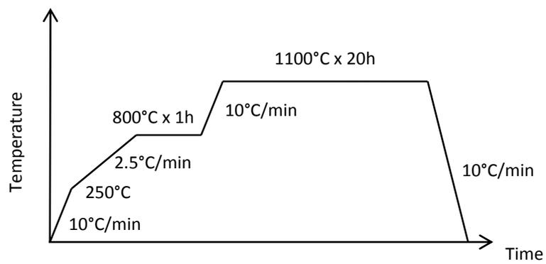
Figure 6: Production of dense  $\beta$ -TCP samples - thermal treatment
