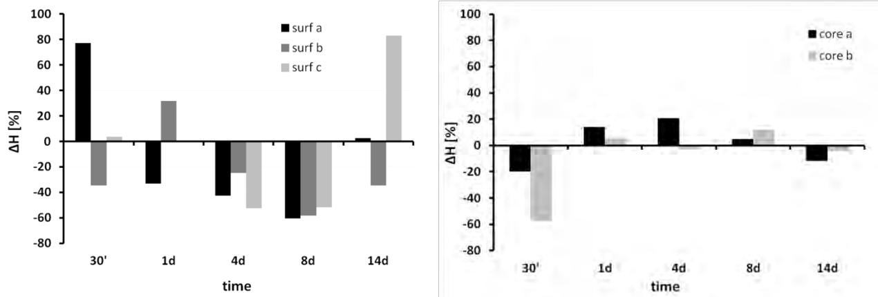
Figure A.b.19: Variation of hardness of DCPD samples at the surface (left) and in the core (right) after different immersion times in TRISd. Average values at  $t_0$ :  $H_{\text{surface}}=9.2\text{MPa}$ ,  $E_{\text{surface}}=1101\text{MPa}$ ,  $H_{\text{core}}=6.1\text{MPa}$ ,  $E_{\text{core}}=882\text{MPa}$
