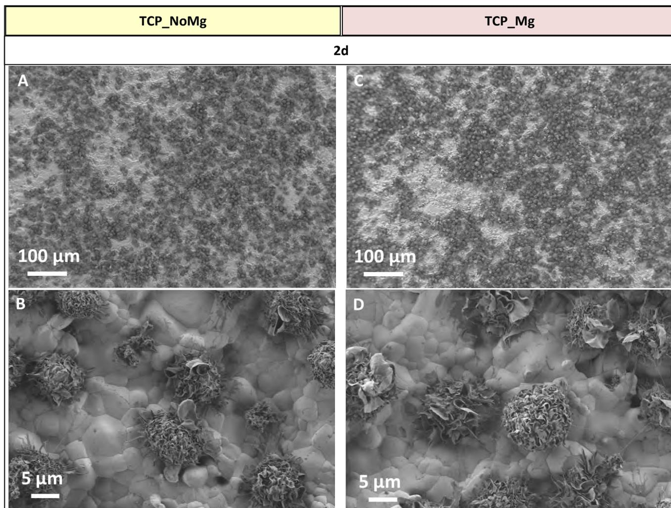
Figure A.d.3: SEM micrographs of cells on  $\beta$ -TCP samples with (C, D) and without (A, B) magnesium after 2 days of culture
