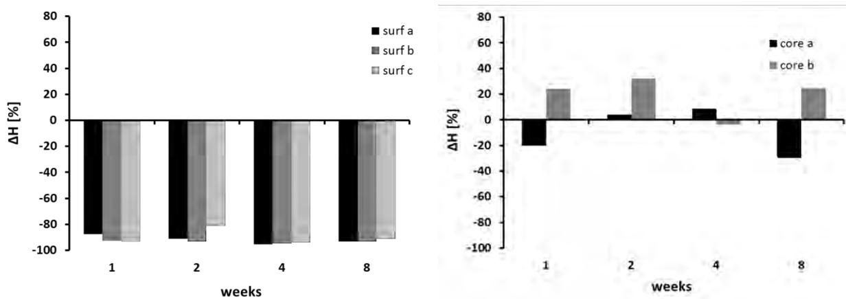
Figure A.c.9: Variation of hardness of  $\beta$ -TCP samples at the surface (left) and in the core (right) after different times of immersion in TRISd. Average values at  $t_0$ :  $H_{surface}=5.0MPa$ ,  $E_{surface}=788MPa$ ,  $H_{core}=3.8MPa$ ,  $E_{core}=986MPa$
