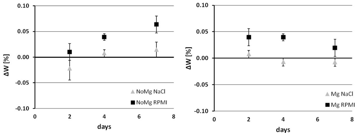
Figure 19: Variations of weight in percentage of pure (left) and Mg-doped (right) samples after acellular dissolution tests. Error bars represent the standard deviation of the measurements. Average weight at time zero: TCP\_NoMg = 0.67 g, TCP\_Mg=0.66 g
