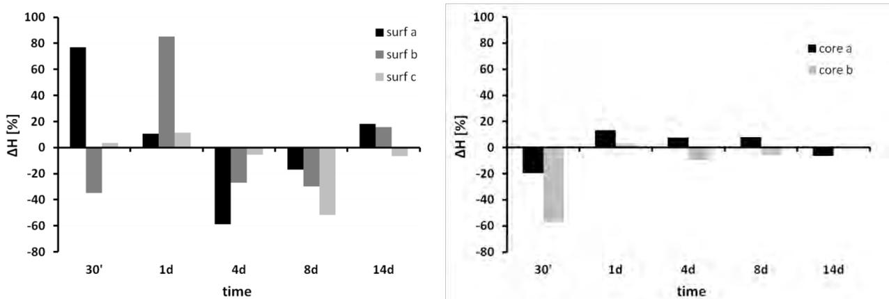
Figure A.b.17: Variation of hardness of DCPD samples at the surface (left) and in the core (right) after different immersion times in TRISs. Average values at  $t_0$ :  $H_{surface}=9.2MPa$ ,  $E_{surface}=1101MPa$ ,  $H_{core}=6.1MPa$ ,  $E_{core}=882MPa$
