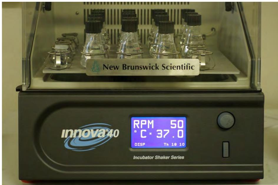
Figure 8: Incubator used for static dissolution tests
