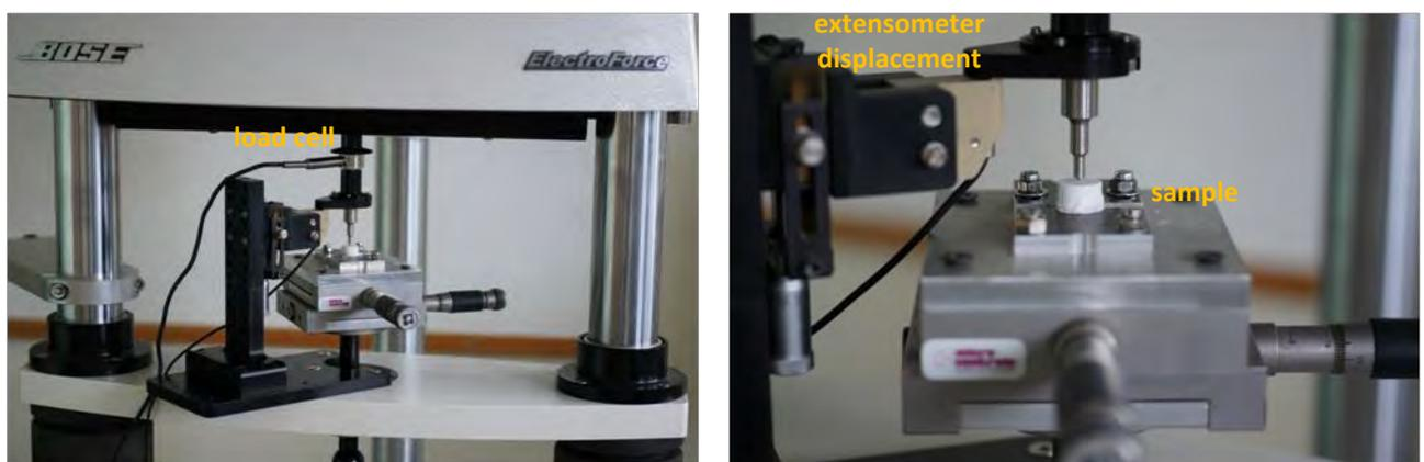
Figure 14: Electroforce® 3200 testing machine
