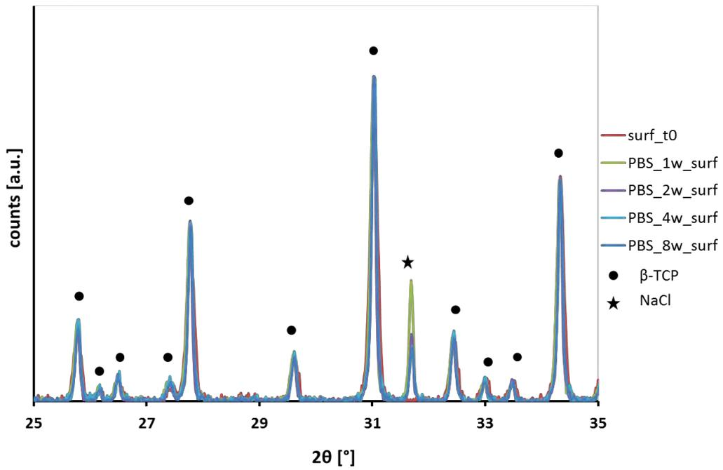
Figure 12: XRD patterns of  $\beta$ -TCP samples at the surface at time 0 and after 1-2-4-8 weeks in PBSd
