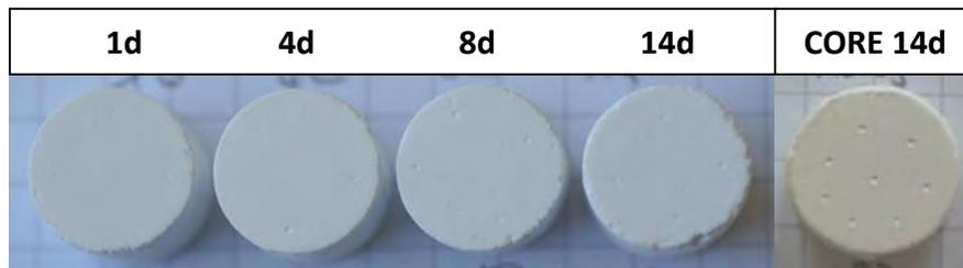
Figure 12: Pictures of samples after immersion in TRISs (dots in the inner part of the section are traces left by the indentation tests)
