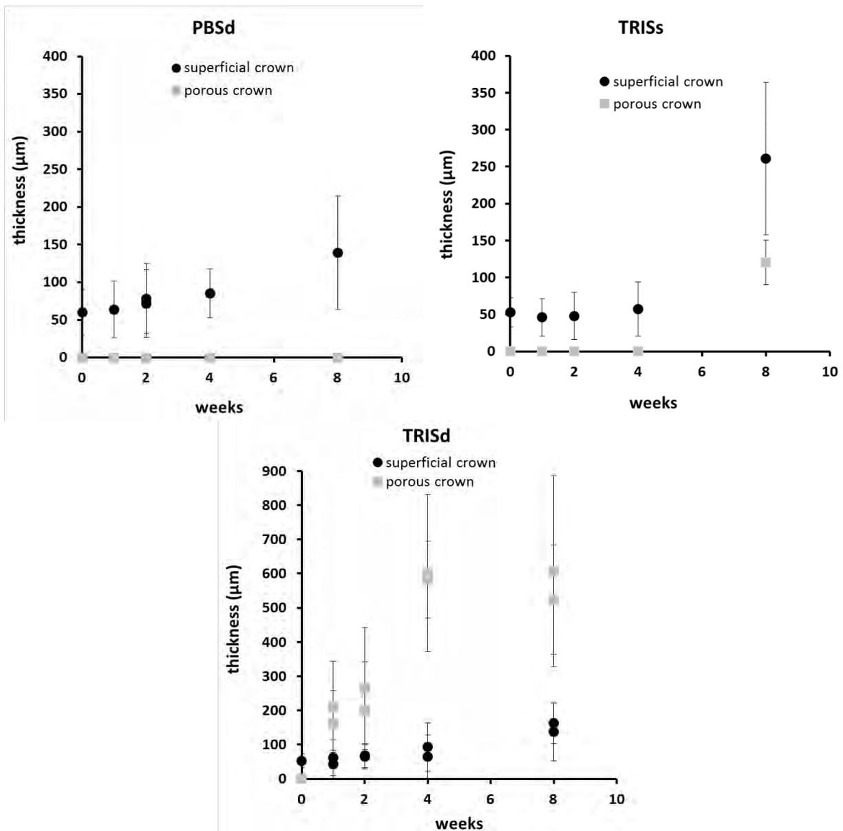
Figure 21: Thickness of layers observed by  $\mu$ -CT in samples after immersion. Notice that the scale of the y-axes in TRISd graph is higher than the one of the graphs of samples immersed in PBSd and TRISs
