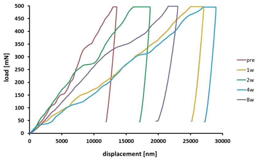
Figure 33: Representative load-displacement curves obtained at the surface of  $\beta$ -TCP samples after immersion in TRISs
