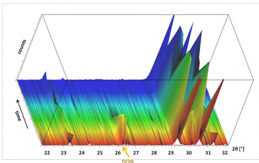
Figure A.b.6: Evolution during time (0-14d) of phases in the core of DCPD samples after immersion in TRISd. Range  $2\theta = 22^\circ - 32^\circ$
