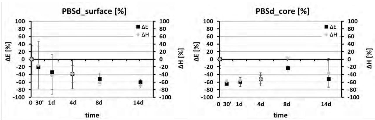
Figure 35: Variation of  $H$  and  $E$  at the surface (left) and in the core (right) after different times of immersion in PBSd
