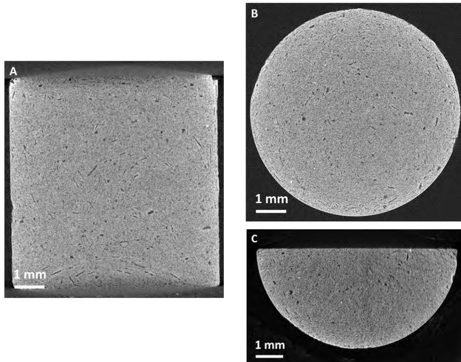
Figure 2: Frontal (A) and transverse (B)  $\mu$ -CT images of an entire cylinder and transverse  $\mu$ -CT image of a half-cylinder (C) of DCPD before immersion (resolution of  $10 \mu\text{m}/\text{voxel}$ )
