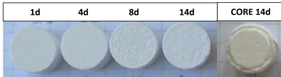
Figure 11: Pictures of samples after immersion in PBSd (dots in the inner part of the section are traces left by the indentation tests)
