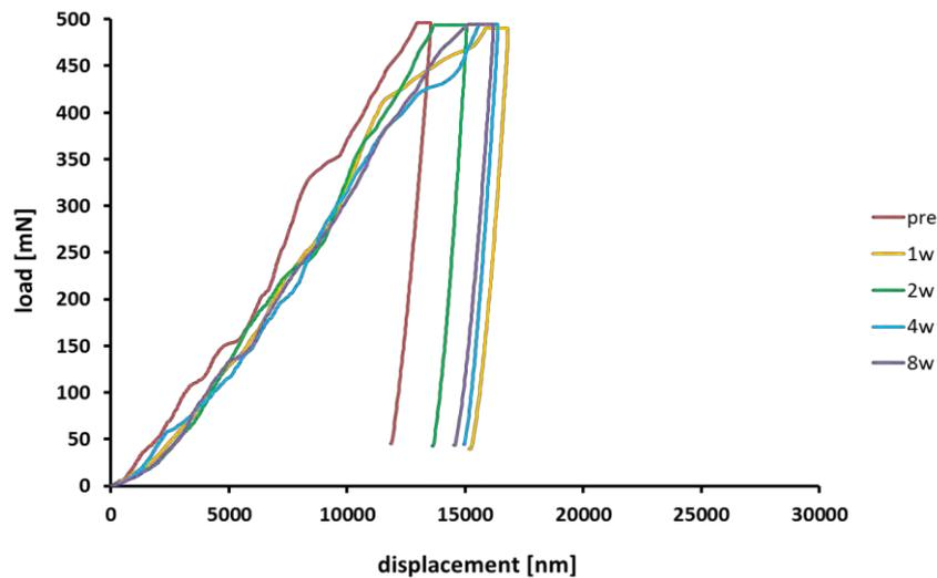
Figure 39: Representative load-displacement curves obtained in the core of  $\beta$ -TCP samples after immersion in TRISd
