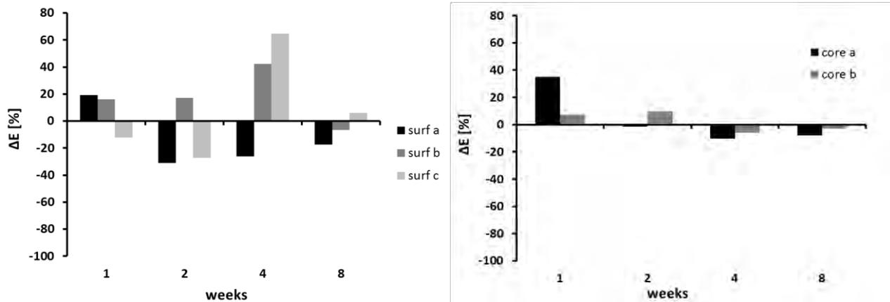
Figure A.c.6: Variation of Young's Modulus of  $\beta$ -TCP samples at the surface (left) and in the core (right) after different times of immersion in PBSd. Average values at  $t_0$ :  $H_{surface}=5.0MPa$ ,  $E_{surface}=788MPa$ ,  $H_{core}=3.8MPa$ ,  $E_{core}=986MPa$
