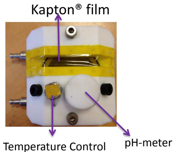
Figure A.b.21: Batch reactor designed for in-situ XRD analyses in liquid media
