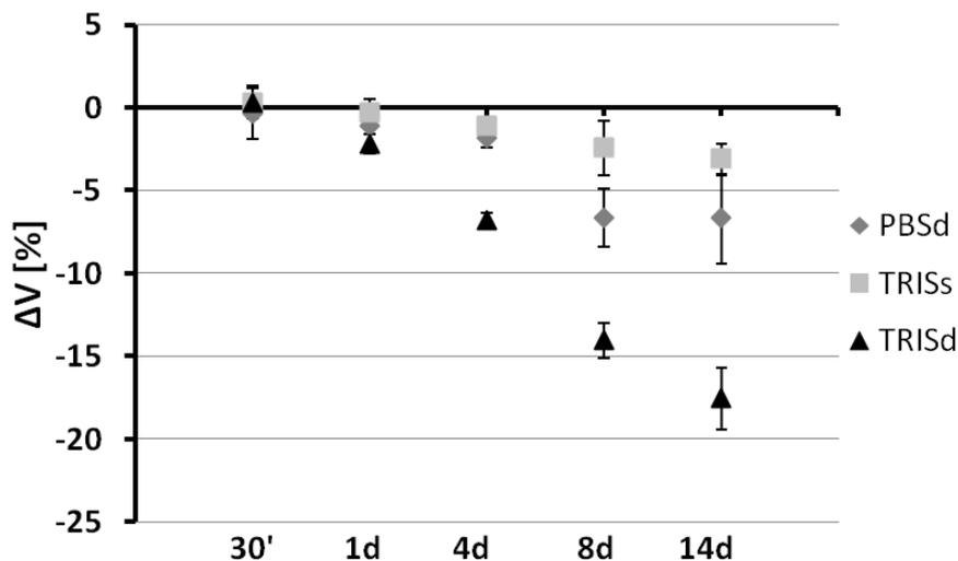
Figure 8: Percent variation of samples volume after immersion (average volume at  $t_0 = 1.37 \pm 0.03$  cm<sup>3</sup>),  $n=3$  ( $n$  being the number of samples per condition)
