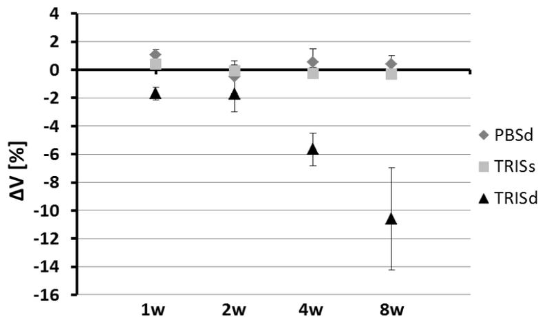
Figure 9: Percent variation of sample volume after immersion (average volume at  $t_0 = 0.6 \text{ cm}^3$ ),  $n=3$  ( $n$  being the number of samples per condition)
