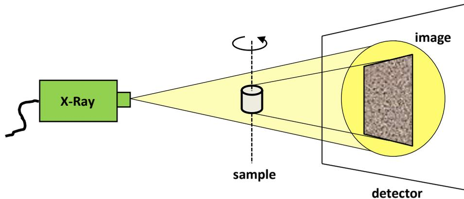
Figure 11: Schematic representation of a X-Ray tomography system
