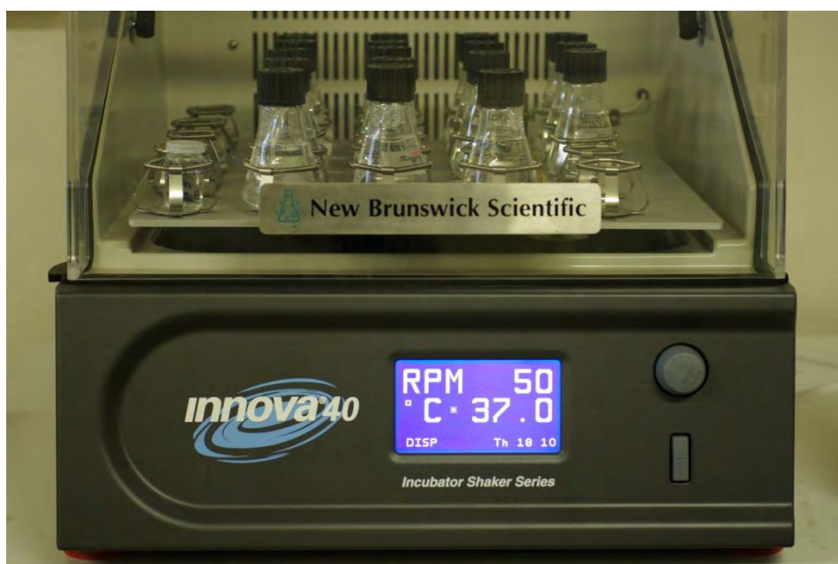
Figure 8: Incubator used for static dissolution tests
