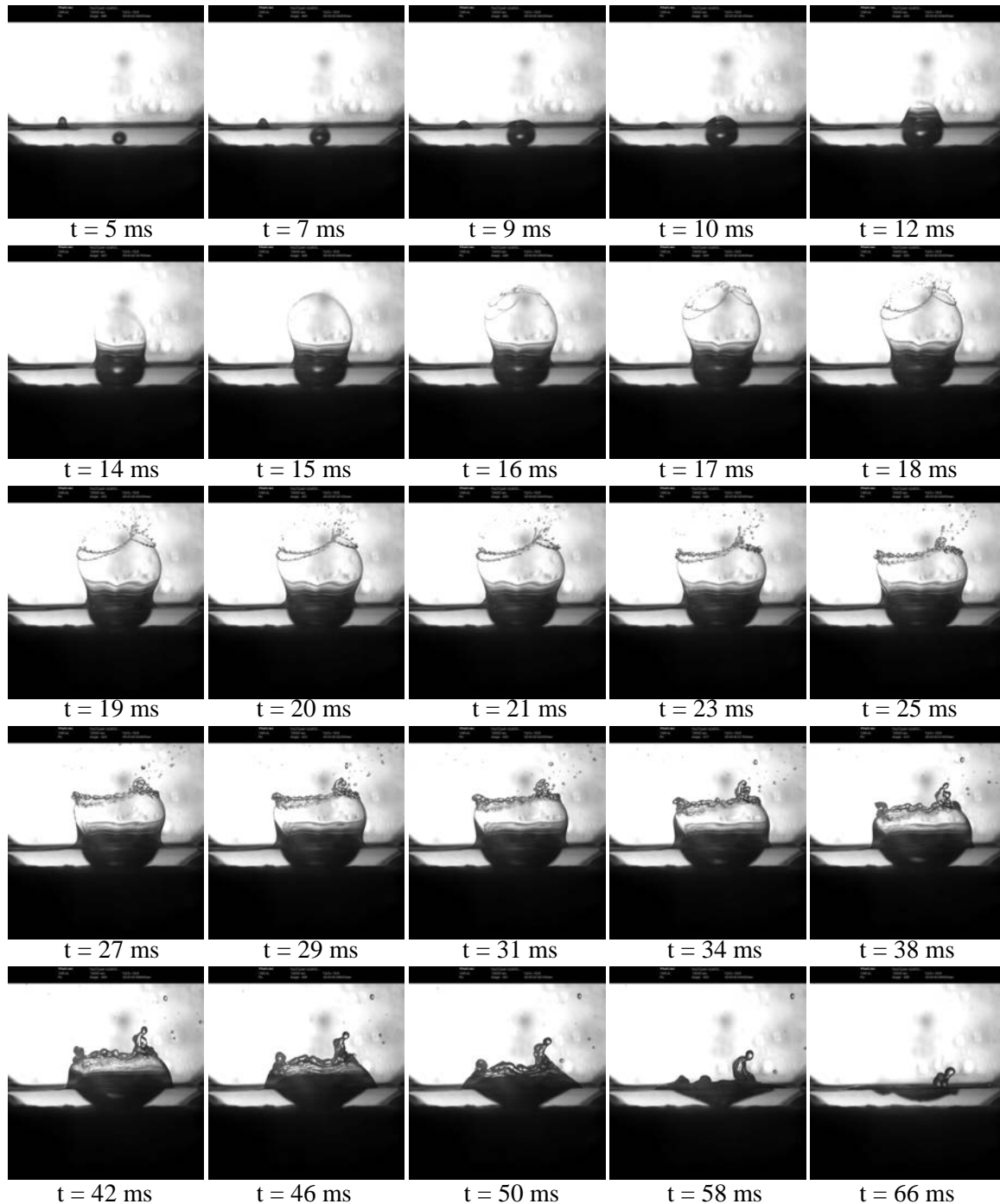
Figure 5.1: Bubble growth in a liquid layer of 3 mm with a breaking of the bubble at the interface liquid/vapor ( P_v = 3 \text{ kPa} , T_1 = 24 \text{ }^\circ\text{C} , h_1 = 3 \text{ mm} , \dot{q} = 1.6 \text{ W.cm}^{-2} )
