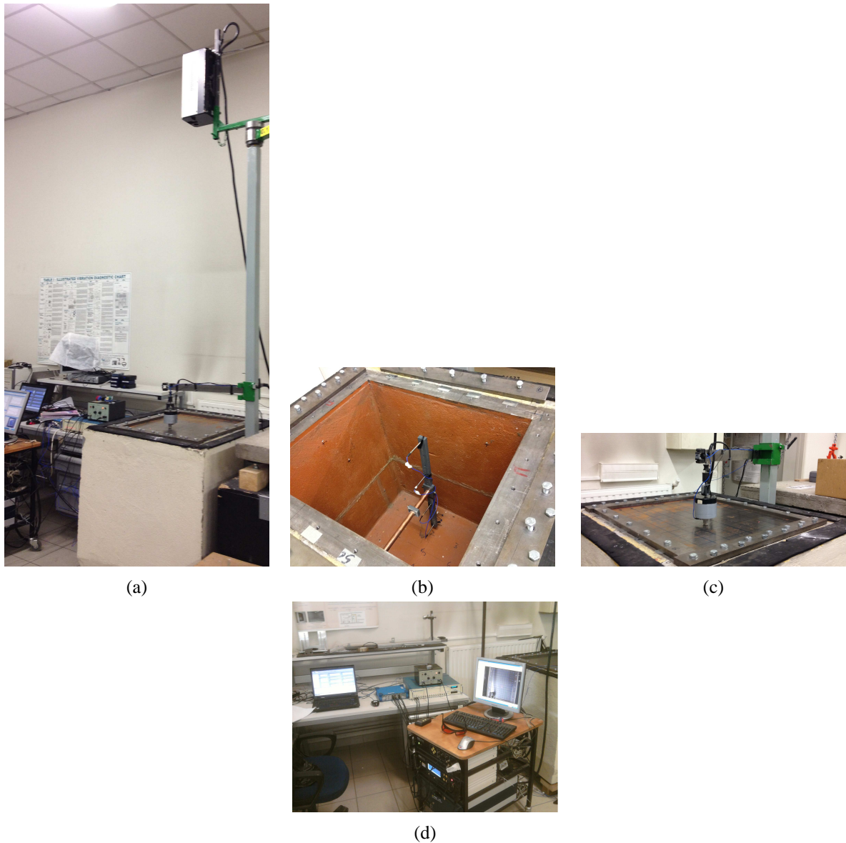
Figure 5.4: Experimental setup: (a) Plate-cavity system and the mounted vibrometer, (b) Mounted microphones inside the cavity, (c) Excitation, (d) Measurement equipment
