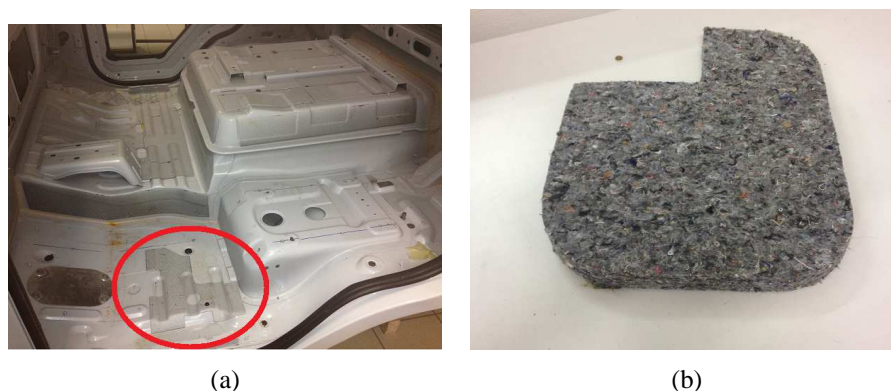
Figure 4.1: Dissipative materials inside Midlum Renault Truck : (a) Viscoelastic damping pad, (b) Composite fibre from the rear surface insulator (membrane in red circle presented in Fig. 3.7a)
