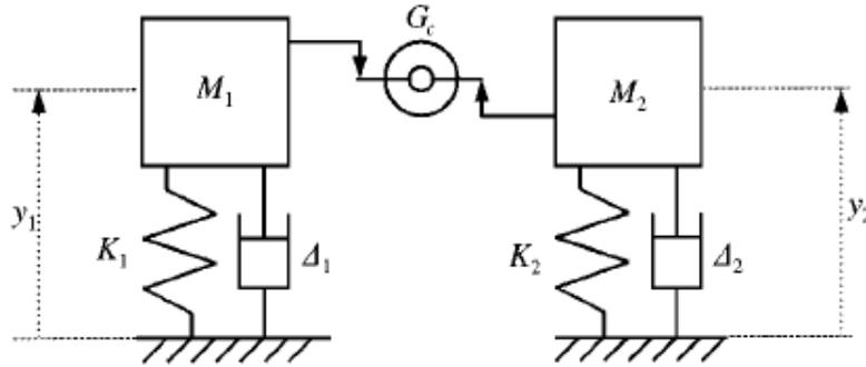
Figure 2.2: Two oscillators coupled by gyroscopic element [60]
