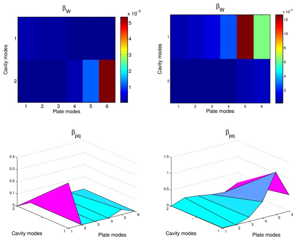
Figure 4.16: The intermodal spectral ( $\beta_W^{12}$ ) and coupling ( $\beta_{pq}^{12}$ ) factors versus coupled resonant modes in 315 Hz band (Modes indexed with increasing natural frequencies): (Left) *Bare*, (Right) *Poro*
