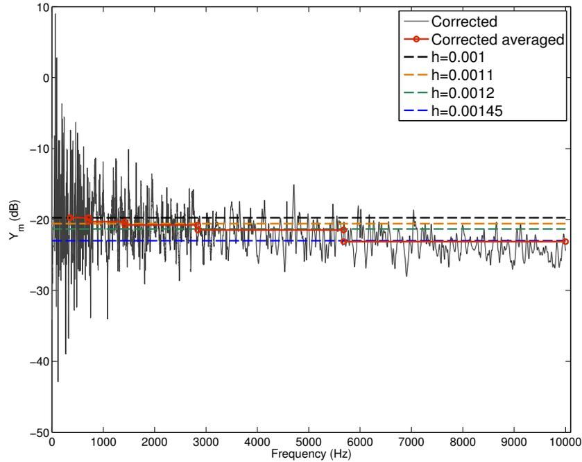
Figure 5.10: Asymptotic values of the input mobility (corrected) of *Bare* plate with respect to a plate thickness (Corrected values in solid  $\circ$  are averaged in an octave band)
