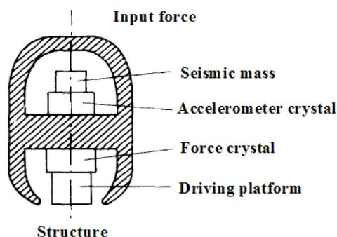
Figure 5.11: Schematic of a typical impedance head design [15]
