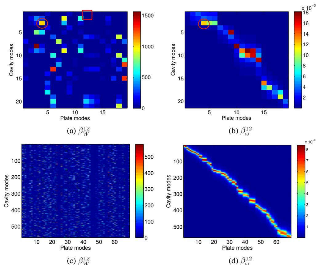
Figure 2.9: The intermodal spatial ( $\beta_W^{12}$ ) and spectral ( $\beta_\omega^{12}$ ) coupling factors versus coupled resonant modes: (Top) 1 kHz band, (Bottom) 3.15 kHz band
