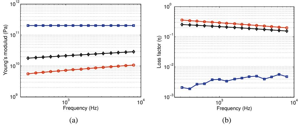
Figure 4.6: Properties of the plate components in 1/3 octave band. The values of the viscoelastic damping pad and the equivalent layer are computed at 20 °C using *MOVISAND* software. ( $\square$ : 1 mm steel plate (*Bare*),  $\circ$ : 3 mm viscoelastic damping pad,  $\diamond$ : 4 mm equivalent layer): (a) Young's modulus, (b) Experimental damping loss factor
