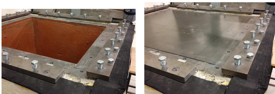
Figure 5.1: Coupling of the plate-cavity system
