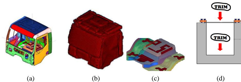
Figure 2: Structure-fluid system (cabin body surfaces and cabin air space): (a) Truck cabin BIW, (b) Cabin air space (3D solid mesh), (c) Cabin floor with trim components (red and blue patches), (d) Plate-cavity system with trim components
