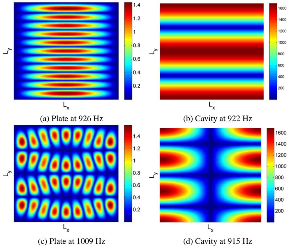
Figure 2.11: Subsystem modeshapes at the coupling surface in 1 kHz band: (Top) Mode couple (3,8) (high  $\beta_W^{12}$  and  $\beta_\omega^{12}$  marked in circles in Fig. 2.9a and 2.9b respectively, and the highest  $\beta_{pq}^{12}$  marked in circle in Fig. 2.10a), (Bottom) Mode couple (12,1) (the lowest  $\beta_W^{12}$  marked in rectangle in Fig. 2.9a)
