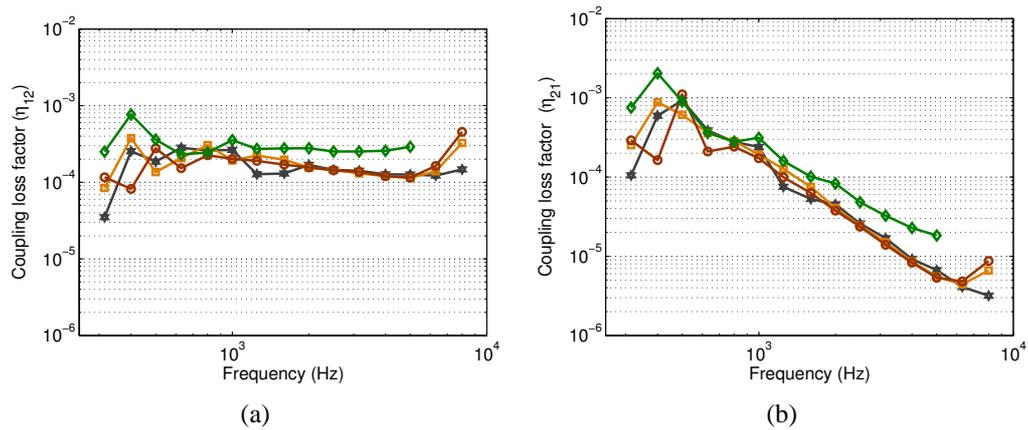
Figure 4.14: Coupling loss factor of each test case in 1/3 octave band ( $\star$ : *Bare*,  $\square$ : *Visc1*,  $\circ$ : *Visc2* and  $\diamond$ : *Poro*): (a) Plate-cavity ( $\eta_{12}$ ), (2) Cavity-plate ( $\eta_{21}$ )
