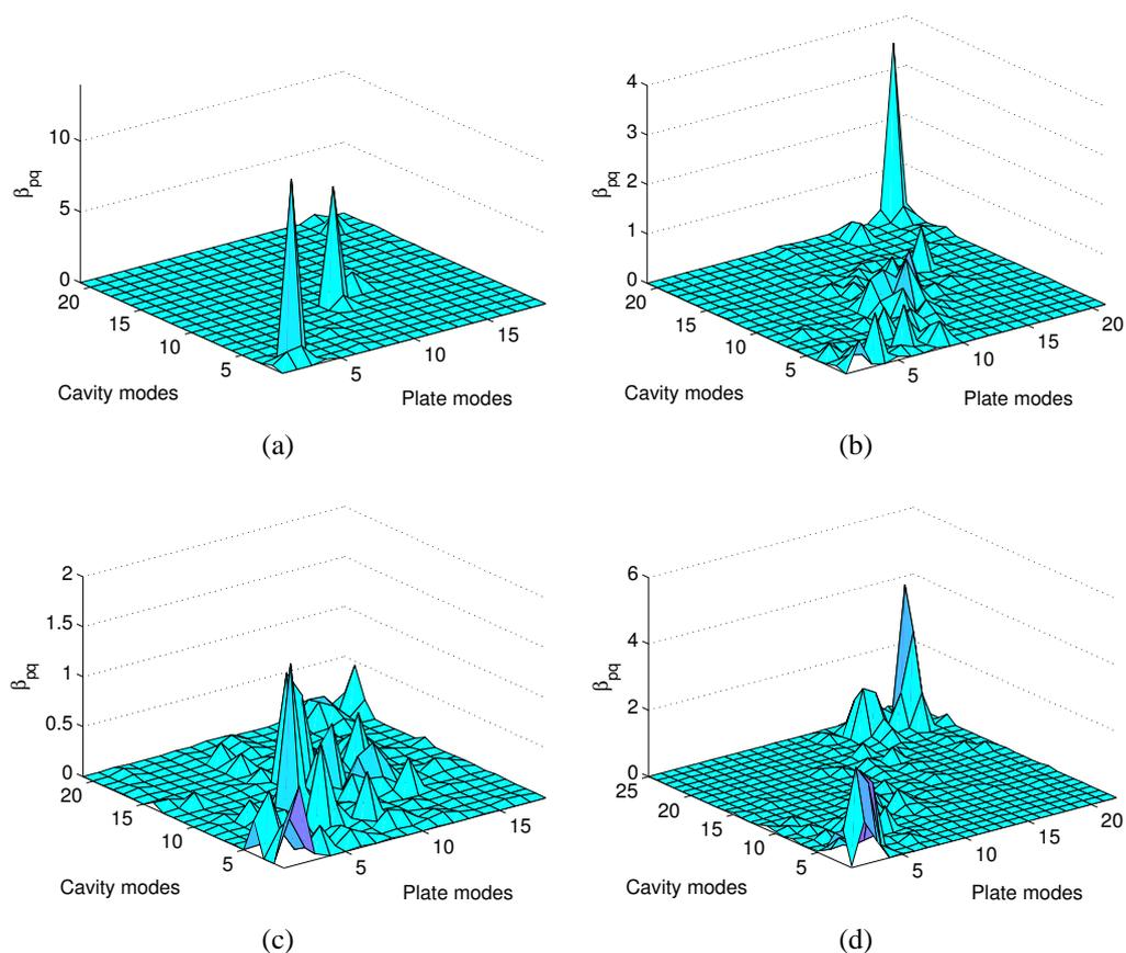
Figure 4.13: The intermodal coupling factors ( $\beta_{pq}^{12}$ ) versus coupled resonant modes in 1 kHz band (Modes indexed with increasing natural frequencies): (a) *Bare*, (b) *Visc1*, (c) *Visc2*, (d) *Poro*
