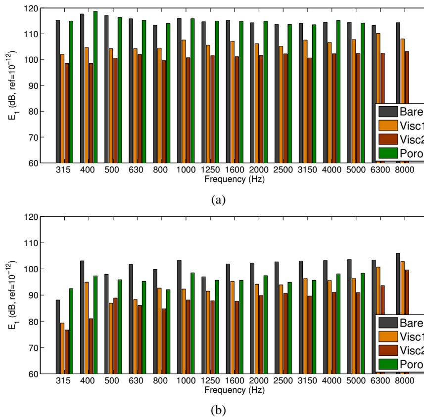
Figure 4.15: Subsystem energies of all test cases in 1/3 octave band: (1) Plate energies, (2) Cavity energies amount of reduction to plate energies. Energies of *Visc1* are reduced by an average 7.5 dB in all frequency
