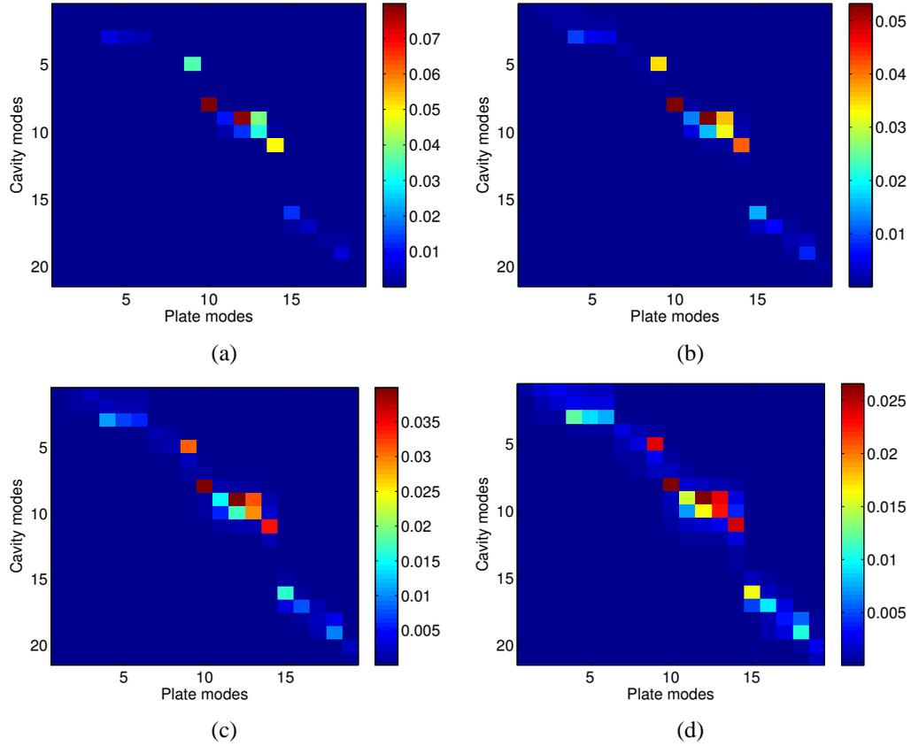
Figure 2.15: The intermodal spectral ( $\beta_{\omega}^{12}$ ) coupling factors versus coupled resonant modes with respect to the plate damping: (a)  $\eta_1 = 0.001$ ,  $\eta_2 = 0.001$ , (b)  $\eta_1 = 0.002$ ,  $\eta_2 = 0.001$ , (c)  $\eta_1 = 0.003$ ,  $\eta_2 = 0.001$ , (d)  $\eta_1 = 0.005$ ,  $\eta_2 = 0.001$
