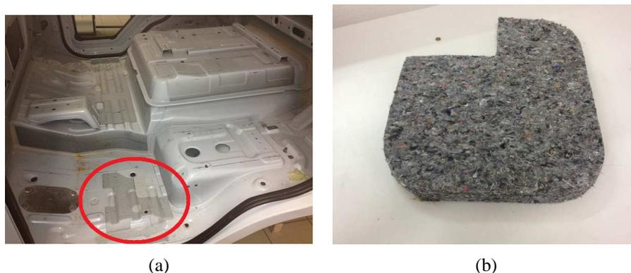
Figure 4.1: Dissipative materials inside *Midlum Renault Truck*: (a) Viscoelastic damping pad, (b) Composite fibre from the rear surface insulator (membrane in red circle presented in Fig. 3.7a)
