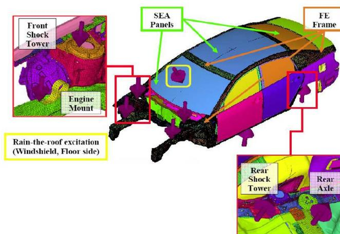
Figure 1.3: Automobile application for Hybrid FE-SEA [23]
