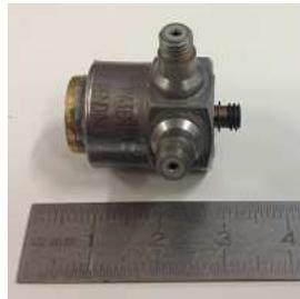
Figure 5.5: PCB 288D01 Impedance head
