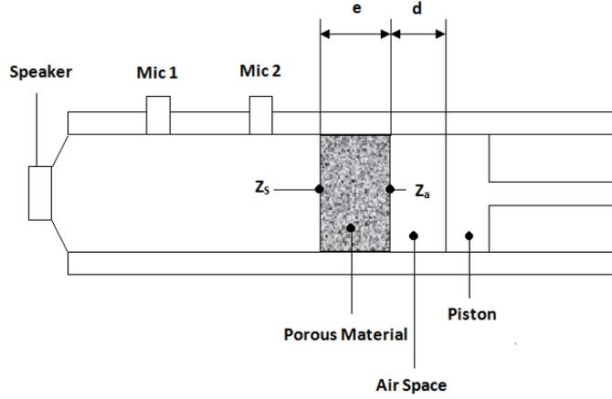
Figure 3.6: Impedance tube measurement of the "Two-cavity method" [85].
