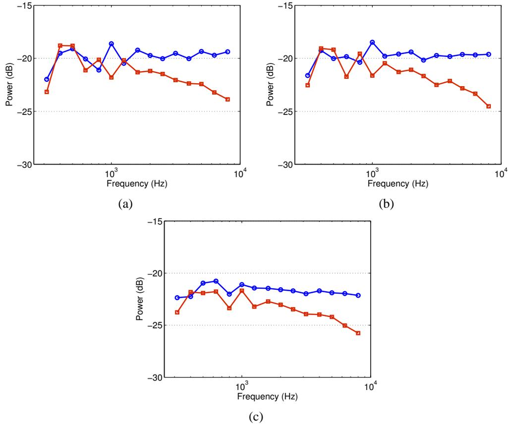
Figure 5.9: The injected power in 1/3 octave band ( $\square$ : experimental,  $\circ$ : numerical): (a) *Bare*, (b) *Visc1*, (c) *Visc2*
