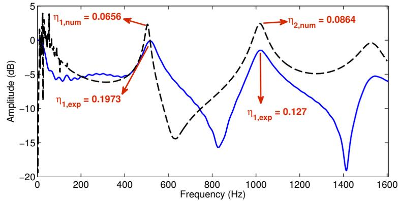
Figure 3.11: Frequency response of the impedance tube terminated by the composite fibre and the modal damping loss factor (Solid: experimental, Dashed: numerical *ACTRAN* software). Amplitudes normalized with the numerical maximum. The damping loss factor is indicated for each resonant peak.
