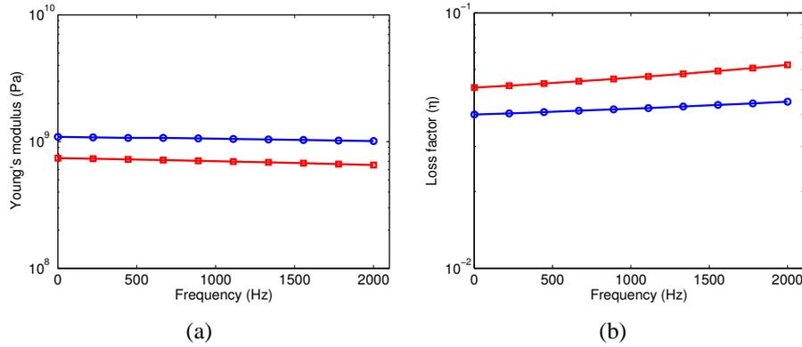
Figure 3.2: Equivalent parameters in a constant frequency band ( $\Delta f=222$  Hz) for the aluminum-PVC composite panel estimated using *MOVISAND* software ( $\circ$ : aluminum + PVC 3 mm,  $\square$ : aluminum + PVC 3.6 mm): (a) Young's modulus, (b) Material loss factor
