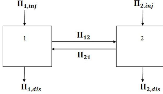
Figure 2.1: A two-subsystem SEA model
