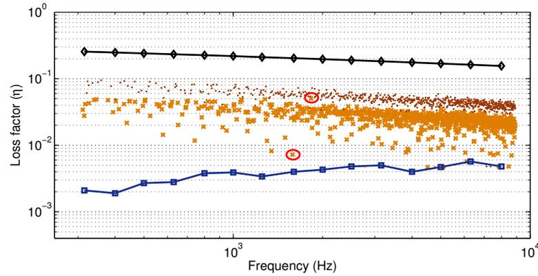
Figure 4.7: The damping loss factor ( $\diamond$ : 4 mm equivalent layer,  $\square$ : experimental result of the steel plate (*Bare*) averaged in 1/3 octave band,  $\times$ : modal values of *Visc1* plate estimated with MSE,  $\bullet$ : modal values of *Visc2* plate estimated with MSE)
