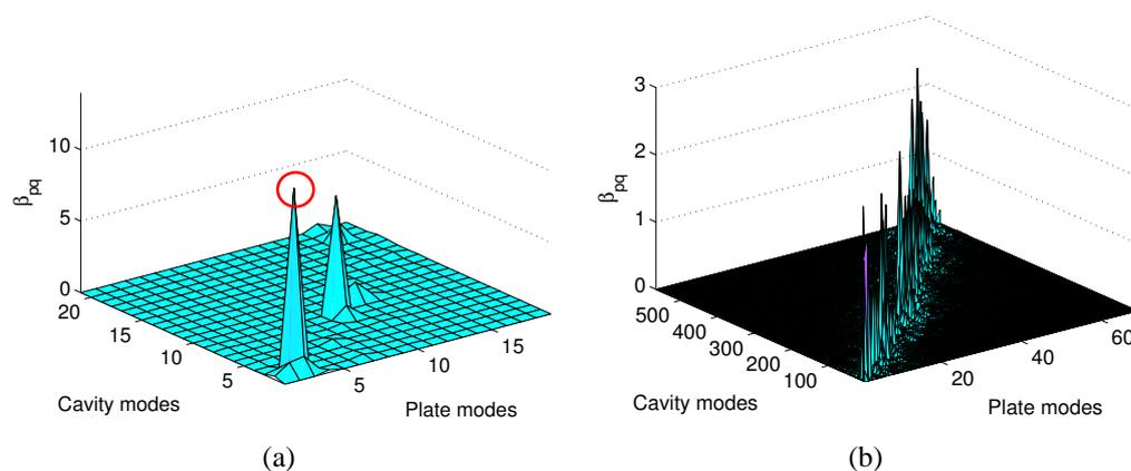
Figure 2.10: The intermodal coupling factors ( $\beta_{pq}^{12}$ ) versus coupled resonant modes (Modes indexed with increasing natural frequencies): (a) 1 kHz band, (b) 3.15 kHz band
