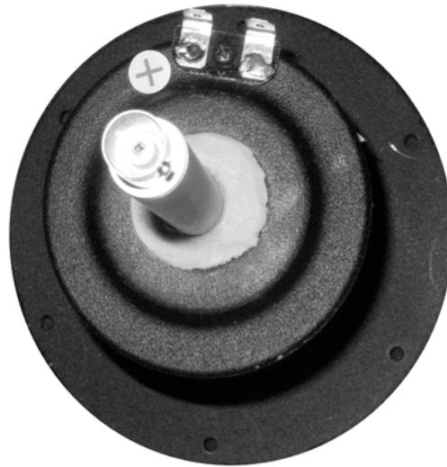
Figure 1: View of the implemented driver's back enclosure equipped with a fixated reference microphone.
