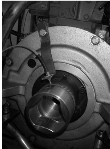
Figure 11: The diesel engine's speed was monitored from the crankshaft rotation using zebra tape and an optical encoder.
