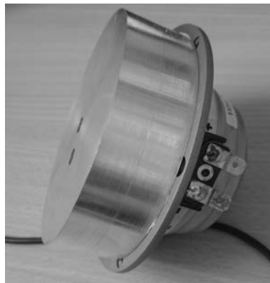
Figure 10: A driver connected to a small cavity was used to calibrate the measurement microphones against a reference microphone.
