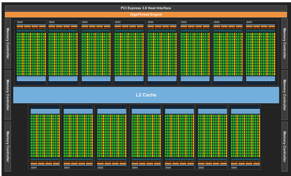
Figure 1.4 – Full Block Diagram of a NVIDIA Kepler GK110.
