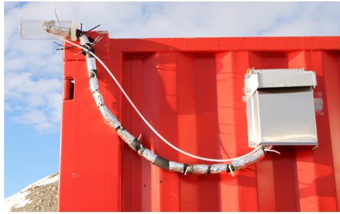
Figure 7.5: The inlet for atmospheric air during the measurement campaign. The coated tubing was heated to 50°C and thermally insulated. A plastic cover around the inlet avoided perturbations because of snow fall
