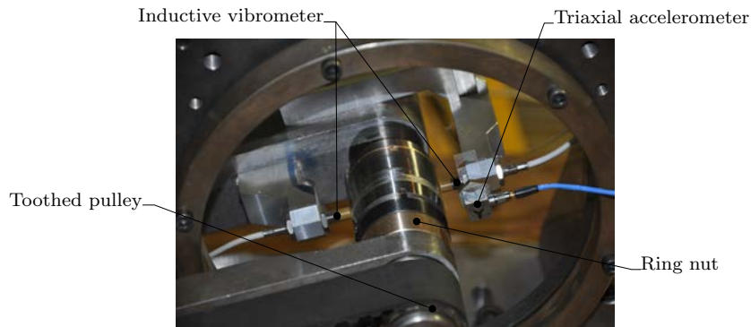
Figure 4.8: Acquisition sensor placement for squeal measurement.
