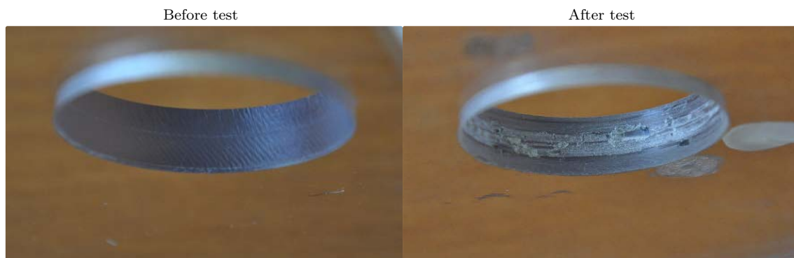
Figure 4.14: Surface status before and after tests of a specimens used in the tests for squeal reproduction, show a rich presence of third body.
