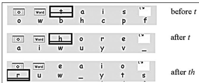
Figure 2. Rearrangement of dynamic keyboard (central part of keyboard shown). (English version of Sibylle.)
