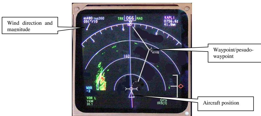
Figure 3.7: Navigation Display (ND) – Boeing term. Indicates the aircraft track, waypoints / pseudo-waypoints and other navigation information [Wikipedia, 2015a]
