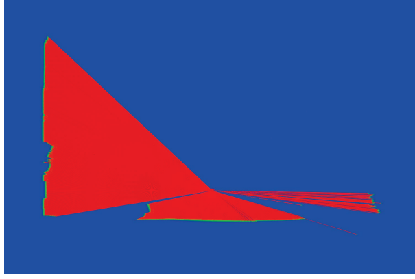
Figure 3.11 – An example of ray occupancy fusion (red: empty, green: occupied, blue: unknown).
