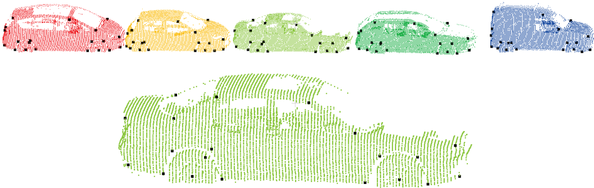
Figure 5.2 – Landmark selection from training samples (one enlarged sample below; landmarks in black). 20 points are selected in total: 16 on one side of the car, one on the wheel edge, two on wheel centres, and one on the other side.
