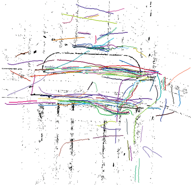
Figure 4.10 – Pedestrian flow in a public place. Pedestrian trajectories are in random colors, and the background is in black.
