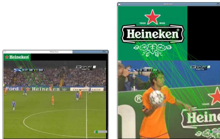
FIGURE 2.3: Two examples of the key-point matching technique using SIFT feature (extracted from [25])
