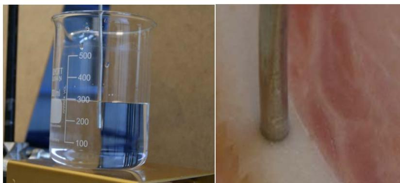
Figure 2.11: Coaxial probe's extremity should contact well with the measured materials
