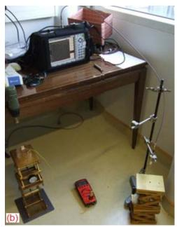
Figure 2.10: Dielectric characterization system for (a) liquid and (b) biological tissue measurements
