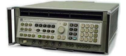
The 8340A synthesized sweepers deliver the combined high-performance of a broadband sweep oscillator in one instrument that is completely controllable via the interface bus. This efficient combination of performance and versatility is ideal for manual or automatic test systems and in many cases enables the HP 8340A to replace a sweep oscillator, a frequency counter, an RF synthesizer, and a microwave synthesizer.
