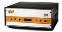
The amplifier of model 25S1G4A produced by Amplifier Research is a solid state, self-contained, air-cooled, broadband amplifier designed for applications where instantaneous bandwidth, high gain and linearity are required. The 25S1G4A, when used with a sweep generator, will provide a minimum of 25 watts of RF power. Included is a front panel gain control which permits the operator to conveniently set the desired output level.
