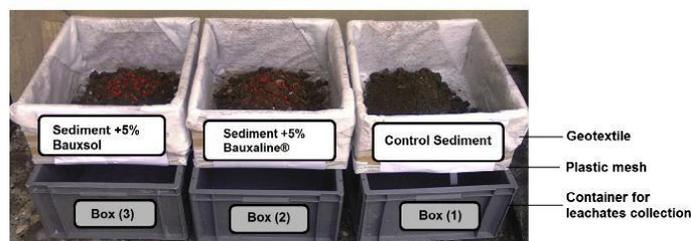
Fig. 1. Experimental setup.
