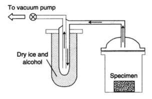
Figure I. 14. Technique de séchage "D-drying" [70]
