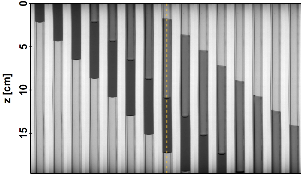
FIGURE 2.2: Image sequence of a typical experiment where a liquid film is deposited at the rear of the liquid slug (light grey). The slug appears in dark grey, V = 2 mL of dyed water. The inner diameter of the polymer tube (PVC) is d_{in} = 6.4 mm. The images are separated by a time step of \Delta t = 0.8 s.
