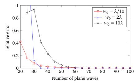
Fig. 2.18 Convergence of incident field with different values of *N* which is the number of plane waves.  $\lambda = 0.1mm$ .
