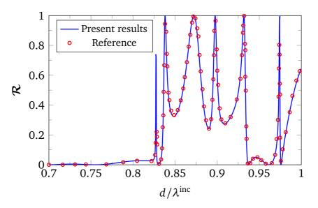
Fig. 4.6 Validating the approach by comparison of the present results (TM polarization) with those of [3].  $\lambda^{\text{inc}}$  is the wavelength of the incident wave.
