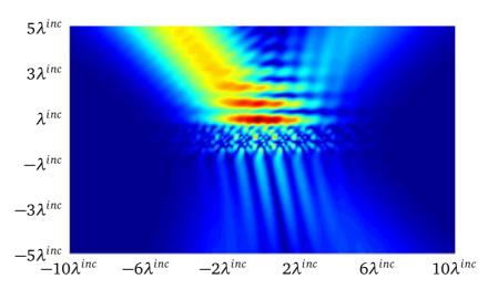
Fig. 2.20 Total field distribution of Gaussian beam scattered by carbon-fiber based slab,  $N = 250, \lambda = 0.1 mm$ .
