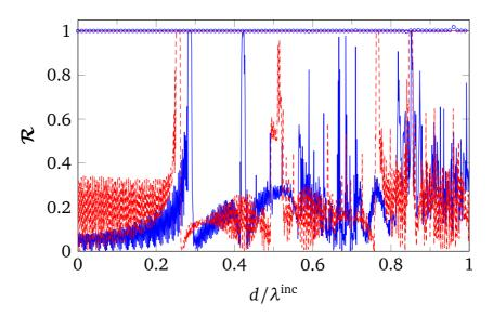
Fig. 4.10 Scattering of a 100-layer composite with epoxy matrix and glass fibers. Plane wave incident normally (dashed, red) or obliquely (solid) with  $\vartheta = 60^{\circ}$  and  $\varphi = 45^{\circ}$ . Energy conservation is checked, and results are shown as straight line (red) for normal incidence and the circles (blue) for oblique case.
