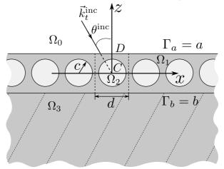
(b) Side view of the structure with transverse components of the incident wave;
