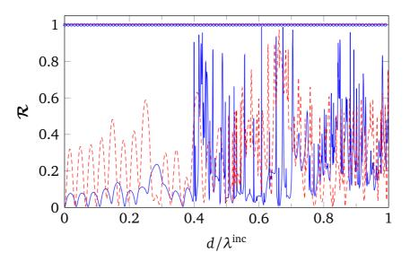
Fig. 4.8 Scattering of an 8-layer composite with alternative background materials and different radius of fibers in different layers, for normally (dashed red curve,  $\vartheta = 0^{\circ}$ ,  $\varphi = 0^{\circ}$ ) and obliquely (solid blue,  $\vartheta = 60^{\circ}$ ,  $\varphi = 45^{\circ}$ ) incident plane waves. Energy conservation is checked, and results are shown as straight line (red) for normal incidence while the circles (blue) for oblique case.
