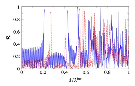
Fig. 5.14 Reflection coefficients of a 32-layer composite consisted of layered 2-layer stacks is given with  $\phi = 60^{\circ}$  for a normally (blue, solid) and obliquely (red, dash dotted,  $\vartheta = 60^{\circ}$ ,  $\varphi = 45^{\circ}$ ) incident E-polarized plane wave.  $d_1 = d_2 = d = 0.1 \text{ mm}$ ,  $h_1 = h_2 = d$  and  $c_1 = c_2 = 0.25d$ .
