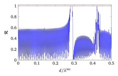
Fig. 5.17 Reflection coefficients of a 100-layer composite consisting of 2-layer stacks with  $\phi = 60^{\circ}$  for E-polarized plane wave with different frequencies. Energy conservation is checked (red solid line).  $d_1 = d_2 = d = 0.1 \text{ mm}$ ,  $h_1 = h_2 = d$  and  $c_1 = c_2 = 0.25d$ .  $\vartheta = 60^{\circ}$ , and  $\varphi = 45^{\circ}$ .
