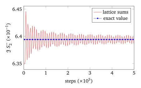
Fig. 2.5 Computed values of  $\Im S_2^-$  with kd = 1.7,  $\alpha_0/d = 1.5$ . The horizontal line represents the exact value 0.639421 calculated with the approach presented in [1]. The partial sums of  $S_m^-$  are computed in steps of 1000, up to  $10^6$ .
