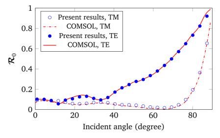
Fig. 2.11 Comparing the present results to the one from COMSOL for TM and TE cases, only the 0-th mode being under consideration.  $d = \lambda_i = 0.1 \text{ mm}$ , L = 2d and c = 0.4d.  $\epsilon_r^{(1)} = 3.6$ ,  $\epsilon_r^{(2)} = 12$ ,  $\sigma_2 = 3.3 \times 10^2 \text{ S/m}$ .
