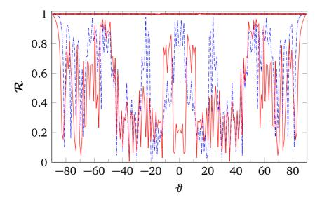
Fig. 5.16 Reflection coefficients of a 100-layer composite consisting of 2-layer stacks with  $\phi = 60^{\circ}$  for E-polarized (dashed, blue) and H-polarized (solid line, red) plane wave. Energy conservation is checked, blue dashed line for E-polarized wave, and red circles for H-polarized one.  $d_1 = d_2 = d = 0.1 \text{ mm}, h_1 = h_2 = d$  and  $c_1 = c_2 = 0.25d$ .
