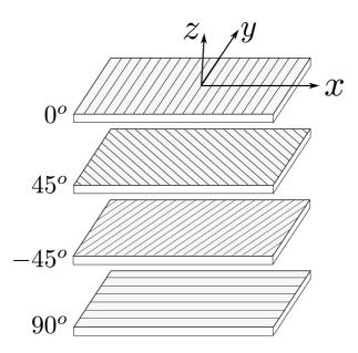
Fig. 5.5 A practical way of fabricating the stack for multilayered composites
