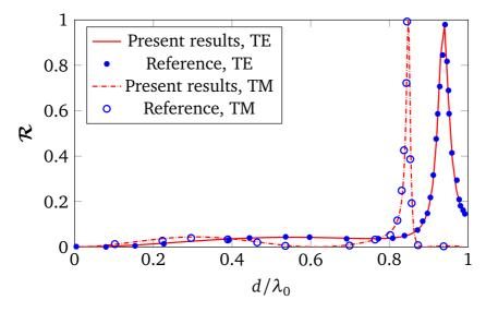
Fig. 2.9 Comparing the present results to the ones of reference [2] for TM wave with c = 0.25d and TE wave with c = 0.375d.  $d = 0.2\mu m$ , L = 0.95d,  $\epsilon_r^{(1)} = 1$ , and  $\epsilon_r^{(2)} = 2$ .
