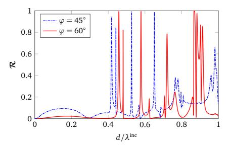
Fig. 3.6 Variation of  $\mathcal{R}$  with  $d/\lambda^{\text{inc}}$ , glass fibers, L = d = 0.1mm, c = 0.25d,  $\vartheta = 60^{\circ}$ .
