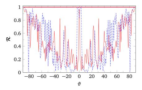
Fig. 5.10 Validating the approach by checking energy conservative law for composite woodpile with  $d/\lambda^{\text{inc}} = 0.5$  (blue, dashed line) and  $d/\lambda^{\text{inc}} = 1$  (red, solid line or circles).
