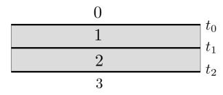
Fig. 5.2 Numbering of the considered laminate and the upper and lower half-spaces;.
