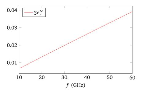
Fig. 2.27 Imaginary parts of effective permittivity of a carbon fiber slab varying with frequency, L = d = 0.1 mm, c = 0.25d, TE wave.
