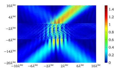
Fig. 4.13 Total field distribution for a Gaussian beam obliquely impinging onto an 8-layer glass-fiber laminate with (0,0) beam center,  $\phi^{inc} = 30^{\circ}$ ,  $\lambda^{inc} = d$ .  $w_0 = 2\lambda^{inc}$ .
