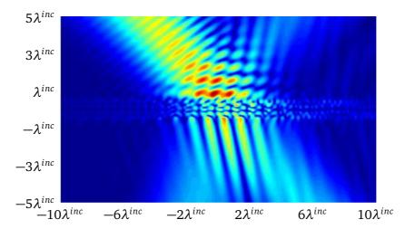
Fig. 2.21 Total field distribution of Gaussian beam scattered by glass-fiber based slab, N = 250,  $\lambda = 0.1mm$ .
