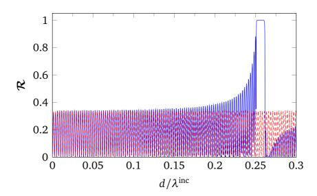
Fig. 4.16 Comparison of the results obtained with homogenized model and exact periodic model under TE wave illumination, normal incidence. Glass-fiber with epoxy background material.  $\lambda^{\text{inc}} = d = 0.1 \text{ mm}, c = 0.25d$ .
