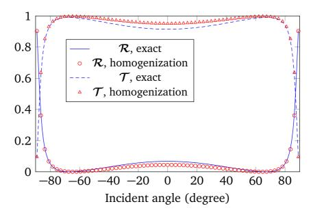
Fig. 2.33 Power reflection and transmission coefficients of a carbon-fiber reinforced slab, L = d = 0.1 mm, c = 0.25d, f = 60 GHz, TE wave oblique illumination.
