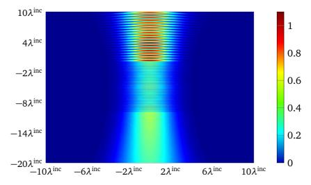
Fig. 4.14 Total field distribution of a Gaussian beam impinging onto a 100-layer model normally, with (0,0) beam center and  $\phi^{inc} = 30^{\circ}$ .  $\lambda^{inc} = 10d$ .  $w_0 = 2\lambda^{inc}$ .
