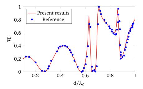
Fig. 2.10 Comparing the present results to the ones of [2] for TM wave with c = 0.375d, and fibers ( $\epsilon_r^{(2)} = 2$ ) are embedded into a slab ( $\epsilon_r^{(1)} = 4$ ) with  $d = 0.2\mu m$  and L = 0.95d.
