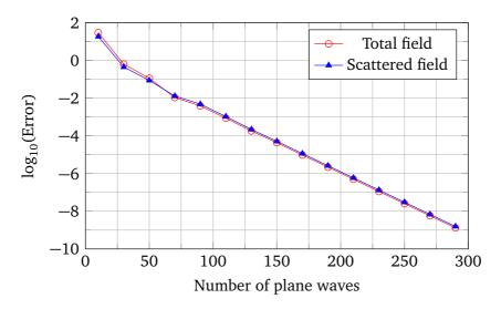
Fig. 2.19 Convergence of scattered field with different values of *N* as the number of planewave components.  $\lambda = 0.1mm$ .
