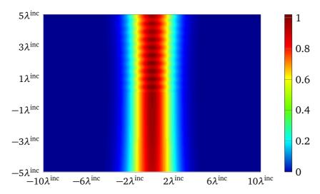
Fig. 2.34 Total field distribution of an E-polarized Gaussian beam normally impinging upon the homogenized slab, L = d = 0.1 mm, c = 0.25d.
