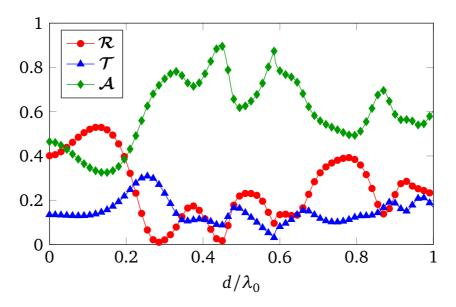
Fig. 2.15 Reflection, transmission and absorption of carbon-fiber based slab under illumination of TM wave.  $\epsilon_r^{(1)} = 3.6$ ,  $\epsilon_r^{(2)} = 12$ ,  $\sigma = 3.3 \times 10^2$  S/m, c = 0.25d. L = d = 0.1 mm.
