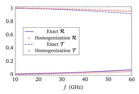
Fig. 2.29 Power reflection and transmission coefficients of a carbon-fiber reinforced slab, L = d = 0.1 mm, c = 0.25d, TE wave normal illumination.
