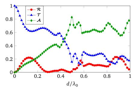
Fig. 2.16 Reflection, transmission and absorption of carbon-fiber based slab under illumination of TE wave.  $\epsilon_r^{(1)} = 3.6$ ,  $\epsilon_r^{(2)} = 12$ ,  $\sigma = 3.3 \times 10^2$  S/m, c = 0.25d. L = d = 0.1 mm.
