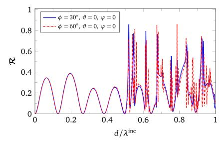
Fig. 5.12 Comparison of results of 2-layer stack with rotation angle of  $\phi = 30^{\circ}$  and  $\phi = 60^{\circ}$ , for normal incident plane wave. Obliquely incident plane is also considered for  $\vartheta = 60^{\circ}$ ,  $\varphi = 45^{\circ}$ .  $d_1 = d_2 = d = 0.1 \text{ mm}$ ,  $h_1 = h_2 = d$  and  $c_1 = c_2 = 0.25d$ .
