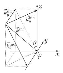
Fig. 5.3 Decomposition of incident wave vector  $\vec{k}^{\text{inc}}$ .
