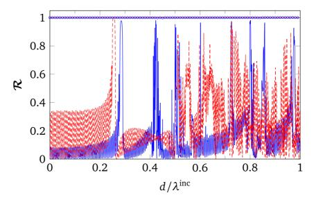
Fig. 4.9 Scattering of a 50-layer composite with epoxy background material. Plane wave incident normally (dashed, red) or obliquely (solid) with  $\vartheta = 60^{\circ}$  and  $\varphi = 45^{\circ}$ . Energy conservation is checked and results are shown as straight line (red) for normal incidence and circles (blue) for oblique case.
