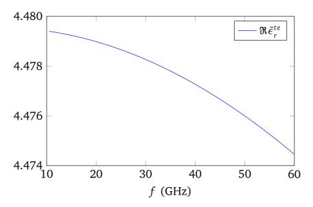
Fig. 2.26 Real part of effective permittivity of a carbon fiber slab varying with frequency, L = d = 0.1 mm, c = 0.25d, TE wave.
