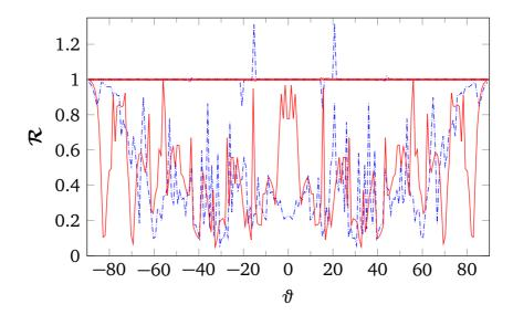
Fig. 5.11 Power reflection coefficients vary with different incident angle for composites constructed with 2 stacks (blue, dashdotted) and 16 stacks (red, solid or circles).  $d/\lambda^{\rm inc} =$  1 for 2-stack composite, and  $d/\lambda^{\rm inc} = 0.5$  for the one with 16 stacks. Each stack has two layers,  $\phi = 60^{\circ}$
