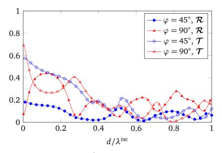
Fig. 3.8 Variation of  $\mathcal{R}$  and  $\mathcal{T}$  with  $d/\lambda^{\text{inc}}$  for  $\varphi = 45^{\circ}$  and  $\varphi = 90^{\circ}$ ,  $\vartheta = 60^{\circ}$ , carbon fibers.
