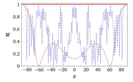
Fig. 5.15 Reflection coefficients of a 100-layer composite made of 2-layer stacks with  $\phi = 60^{\circ}$  for different incident angles, with  $d/\lambda^{\text{inc}} = 0.5$  (blue dashed line) and f = 60 GHz (red solid line), E-polarized plane wave.  $d_1 = d_2 = d = 0.1 \text{ mm}$ ,  $h_1 = h_2 = d$  and  $c_1 = c_2 = 0.25d$ .
