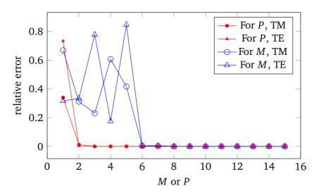
Fig. 2.8 Relative error versus *M* or *P* for glass fibers ( $\epsilon_r^{(2)} = 6.0$ ) embedded in an epoxy matrix ( $\epsilon_r^{(1)} = 3.6$ ).  $d = \lambda_i = 0.1 \text{ mm}$ , L = 2d, c = 0.4d.
