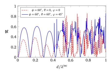
Fig. 5.13 Comparison of results of 2-layer stack with rotation angle of  $\phi = 60^{\circ}$ , for normally and obliquely ( $\vartheta = 60^{\circ}$ ,  $\varphi = 45^{\circ}$ ) incident plane wave.  $d_1 = d_2 = d = 0.1 \text{ mm}$ ,  $h_1 = h_2 = d$  and  $c_1 = c_2 = 0.25d$ .
