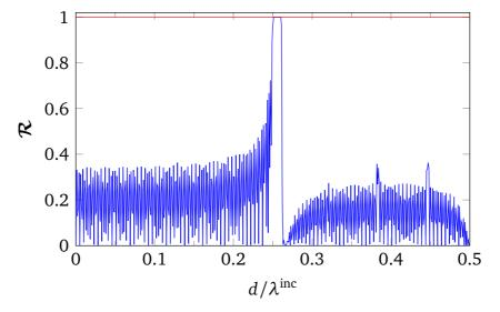
Fig. 5.18 Reflection coefficients of a 100-layer composite constructed with 4-layer stacks is given with  $\phi_1 = 45^\circ$ ,  $\phi_2 = -45^\circ$  and  $\phi_3 = 90^\circ$  for a normally incident E-polarized plane wave. Energy conservation law is checked (red solid line). All layers have the same period  $d_l = d = 0.1 \text{ mm}$ , thickness  $h_l = d$  and radius  $c_l = 0.25d$ .
