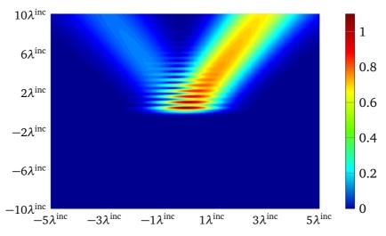
Fig. 4.12 Total field distribution for a Gaussian beam obliquely impinging onto an 8-layer carbon-fiber laminate, with (0,0) beam center and  $\phi^{inc} = 30^{\circ}$ .  $\lambda^{inc} = 10d$ .
