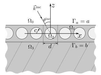
Fig. 2.1 Sketch for the single layer composite structure with TM or TE polarized waves impinging upon it obliquely.
