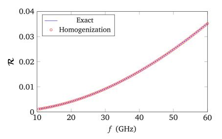
Fig. 2.23 Reflection coefficient of homogenized glass-fiber-based slab for normally incident TM wave, L = d = 0.1 mm, c = 0.25d.
