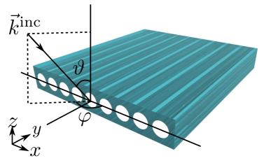
(a) The conically incident electromagnetic plane wave;
