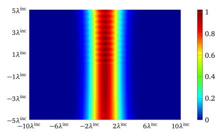
Fig. 2.35 Total field distribution of an E-polarized Gaussian beam normally impinging upon the glass-fiber based slab, L = d = 0.1 mm, c = 0.25d.
