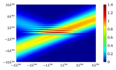
Fig. 4.11 Total field distribution for a Gaussian beam obliquely impinging onto an 8-layer glass-fiber laminate, with (0,0) beam center and  $\phi^{inc} = 45^{\circ}$ .  $\lambda^{inc} = 10d$ .
