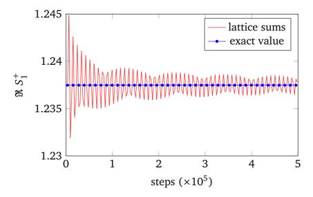
Fig. 2.4 Computed values of  $\Re S_1^+$  with  $k_1 d = 0.7$ ,  $\alpha_0/k_1 = 0.5$ . The horizontal line represents the exact value 1.23746 calculated with the approach given in [1]. The partial sums of  $S_m^+$  are computed in steps of 1000, up to  $10^6$ .
