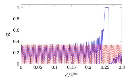
Fig. 4.15 Comparison of the results obtained with homogenized model and exact periodic model under TM wave illumination, normal incidence. Glass-fiber with epoxy background material.  $\lambda^{\text{inc}} = d = 0.1 \text{ mm}, c = 0.25d$ .
