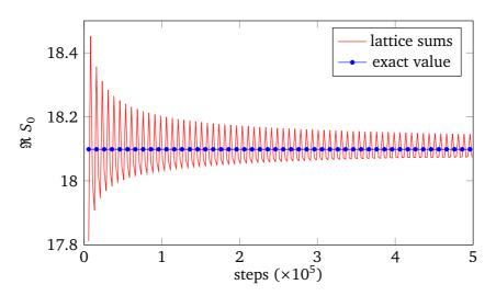
Fig. 2.7 Computed values of the real part of  $S_0$  for f = 5 GHz,  $\theta_i = 0$ , L = d = 0.1 mm. Fast oscillation show up, but it converges slowly.
