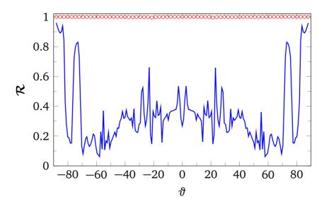
Fig. 4.7 Validating the approach with energy conservation  $\mathcal{R} + \mathcal{T} = 1$  for epoxy matrix with glass fibers.  $\lambda^{\text{inc}}$  is the wavelength of the incident wave, and  $d/\lambda^{\text{inc}} = 1$ . Energy conservation is checked, and results are shown as red circles.
