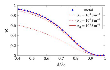
Fig. 2.12 Power reflection coefficients of a periodic array of carbon fibers with multiple conductivities.  $\epsilon_r^{(1)} = 1$ ,  $\epsilon_r^{(2)} = 12$ , c = 0.15d.  $d = 0.2\mu m$ , L = 0.95d, TM incident wave.
