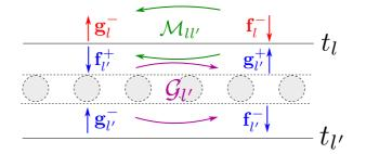
Fig. 4.4 The procedure of calculation from layer to layer with transfer matrices.
