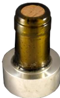
Figure III.3.5: Bottleneck inserted in a metal ring for oxygen transfer measurements
